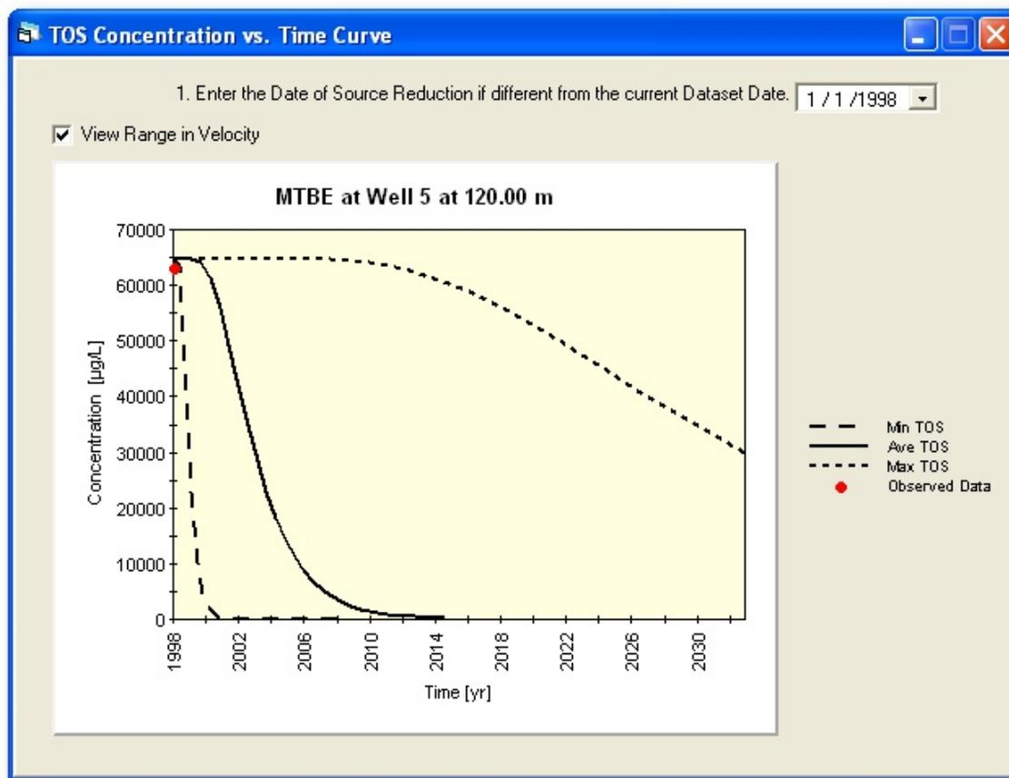
Figure 21. TOS – Graphical Output – Concentration vs. Time
