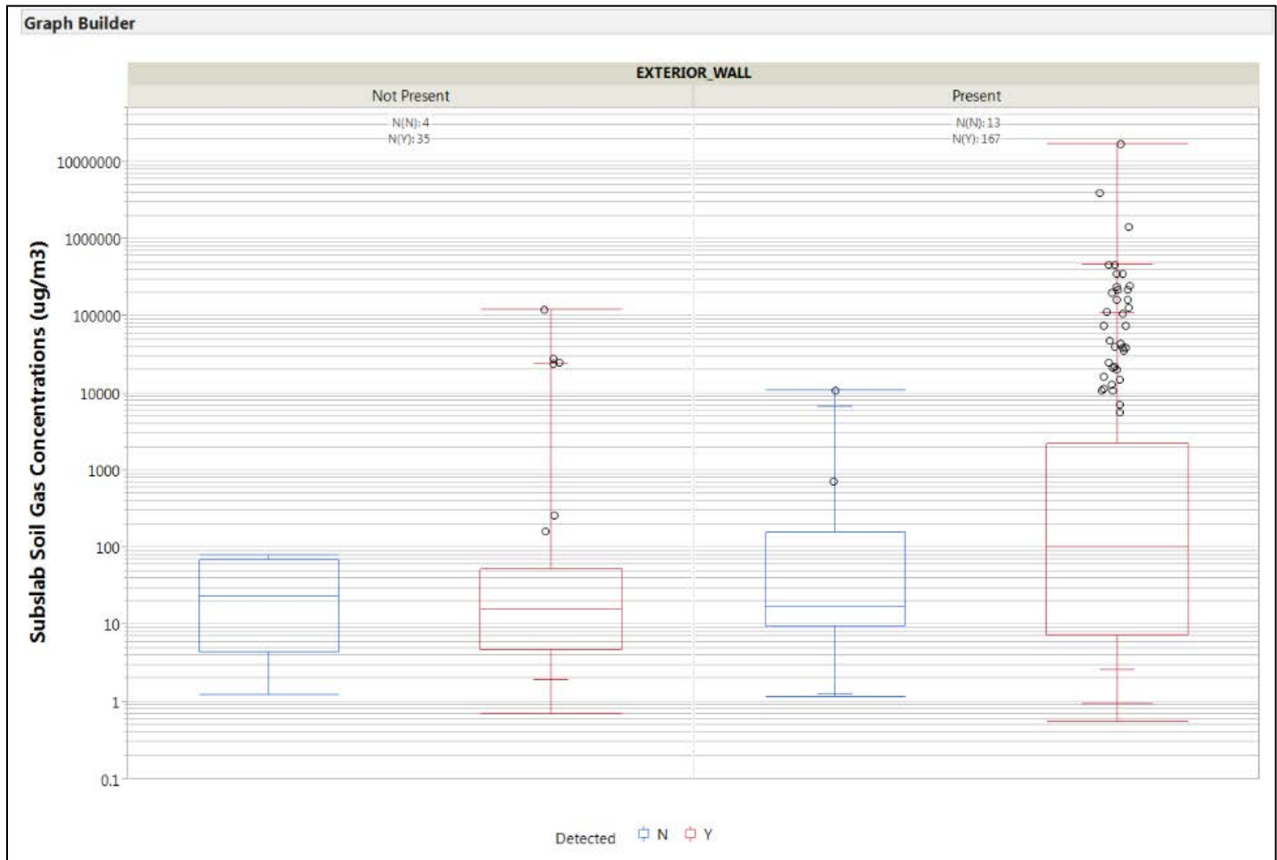
FIGURE E164 PCE Sub-slab Soil Gas Concentration by Exterior Wall Presence NESDI Project #476
