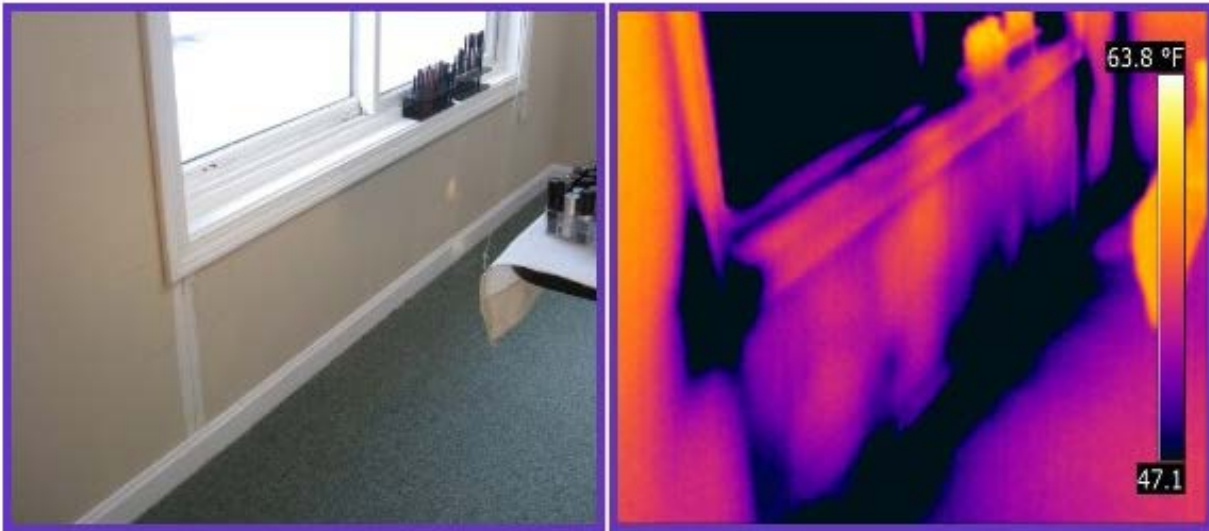
Photograph 6-2: Thermal Camera Image Taken within a Building, Showing how Preferential Heat Flow Occurs at Locations that Appear Visually Well Sealed Reprinted from http://homeenergypros.lbl.gov/profiles/blogs/infrared-imaging-uncovers-many
