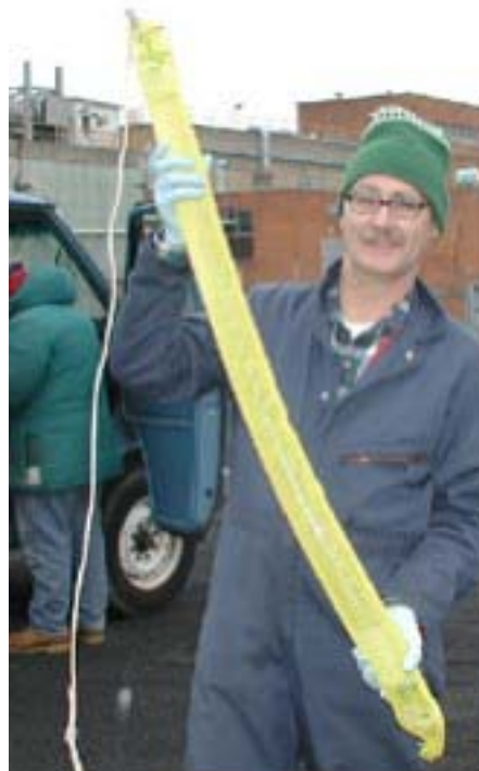
Figure 4-2. Fully constructed dialysis sampler (~ 2.5 inches in diameter by 48 inches long)
