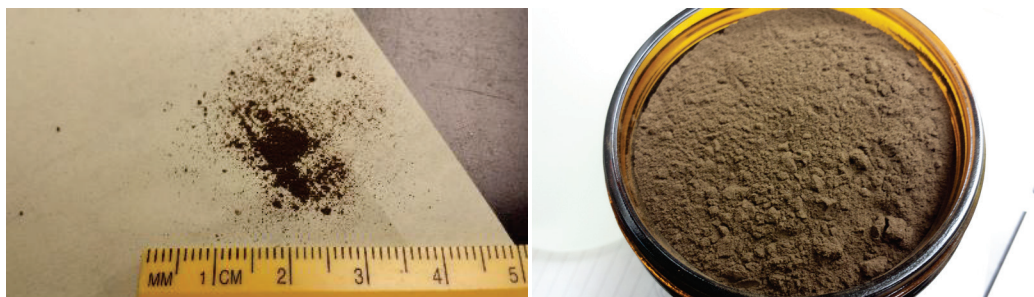
Figure 11. Very fine, homogenized soil used in the explosives study.
