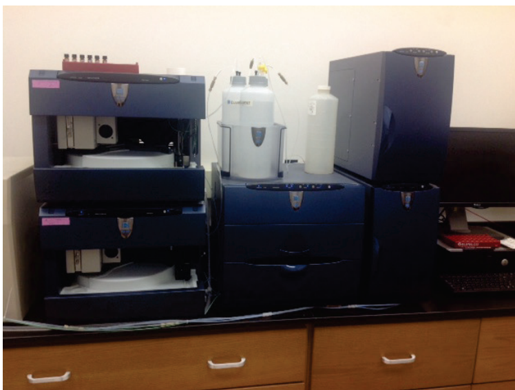
Figure 12. Dionex ion chromatograph used for analysis of inorganic nitrogen species.
