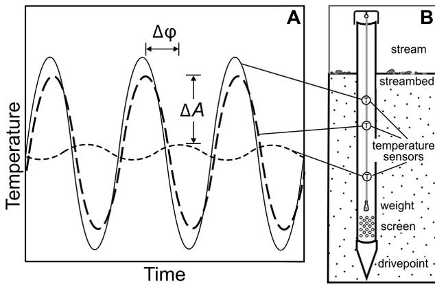
**Figure 3.** (a) Three hypothetical streambed thermographs graphed over three days, showing phase shift ( $\Delta\phi$ ) and difference in temperature amplitude ( $\Delta A$ ), and (b) a typical temperature acquisition assembly inside a piezometer (modified from Hatch *et al.* [2006]).
