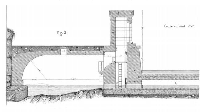
**Figure 2.** Section of Rosoir Spring Inlet Structure, covered aqueduct on the right. Detail from *Darcy* [1856, Plate 3].
