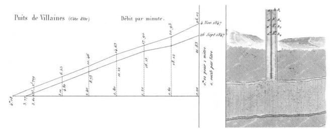
Figure 4. Spring flow measurements. Detail from *Darcy* [1856, Plate 22].
