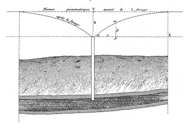
**Figure 7.** Dupuit's solution for radial flow [*Dupuit*, 1863, Figure 69] (History of Hydraulics Collection, Iowa Institute of Hydraulic Research).
