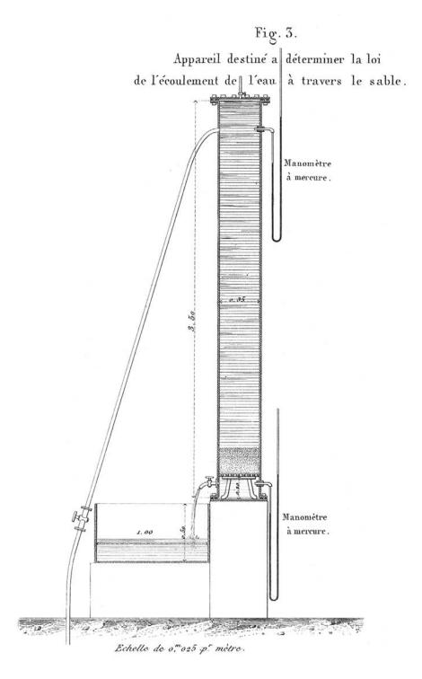
**Figure 5.** Column apparatus [*Darcy*, 1856, Figure 3, Plate 24].
