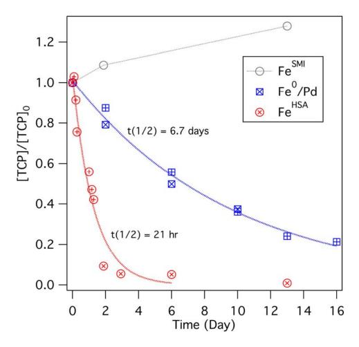
Figure 8. Results of batch experiments done with TCP and several alternative heterogeneous reductants. Fe $^{\text{SMI}}$  is SMI-III from North American Hoganas, Fe $^{\text{HSA}}$ , is HC-15 from Hepure Technologies, and Fe $^{\text{O}}$ /Pd synthesized at OHSU.
