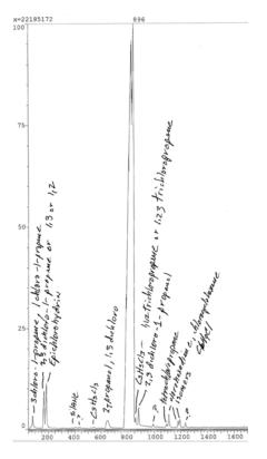
Figure 2. Sample total ion chromatogram from total GC/MS. Note that Fenton reaction--presumably like other oxidants used in ISCO—degrades TCP to a complex mixture of oxygenated and relatively polar products.
