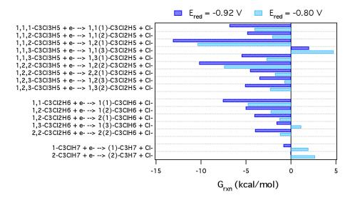
Figure 9. Free energies for dissociative electron transfer (dechlorination) calculated with B3LYP. All chlorinated congeners of propane are included. Two sets of free energies are shown: one for a strong reductant like Fe<sup>0</sup> (with standard reduction potential = -0.92 V) and the other for a more mild reducing agent (with standard reduction potential = -0.80 V) Calculations performed by Eric Bylaska (Pacific Northwest National Laboratory).
