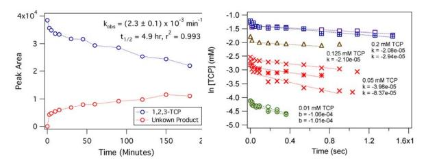
Figure 17. Results from batch experiments under classic Fenton conditions. (1,2,3-TCP = 0.05 mM,  $H_2O_2$  = 300 mM,  $FeCl_2$  = 25 mM, pH = 2.9, T = 25°C).
