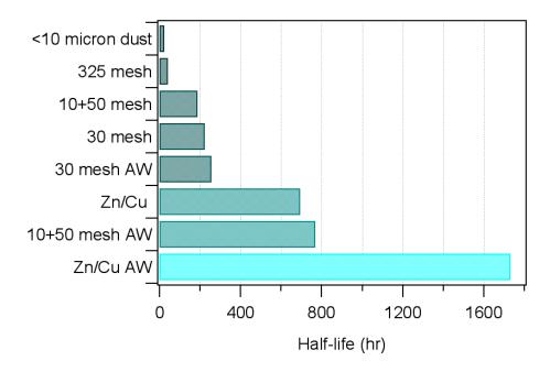
Figure 10. Disappearance rates (plotted as half-lives) for eight types zinc power in DI Water. These data are not corrected for differences in surface area. "Zn/Cu" is bimetallic Cu on Zn. "AW" stands for acid washed.
