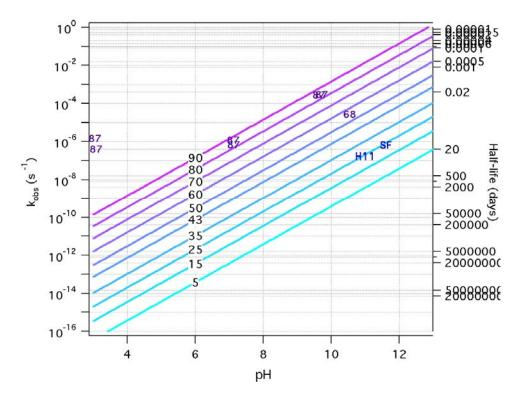
Figure 4. Hydrolysis rate constants vs. pH and temperature calculated from rate constants given in (6). Superimposed are individual data points from (5) (shown as numbers for their respective temperatures), and our data for pH 11 carbonate buffer (labeled H11), and 5 mM  $Na_2S$  at pH = 11.6 (labeled SF).
