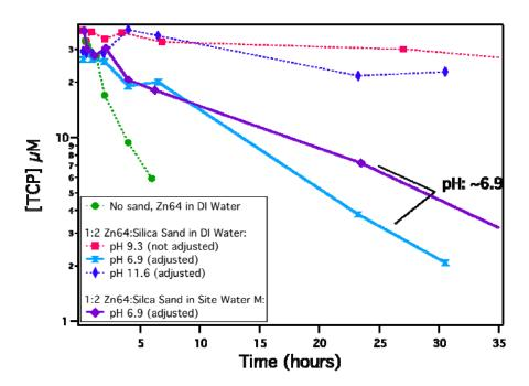
Figure 33. Comparison between batch kinetics of reactors containing ZVZ and sand in DI water and site water at low pH. The curves for 1:2 Zn64:Silica Sand in pH 6.9 DI water and pH 6.9 site water look nearly identical. This result suggests that the inhibition caused by site water and sand are not additive.
