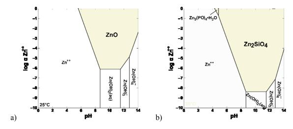
Figure 42. Solubility diagrams for  $Zn^{2+}$  species in (**A**) DI water and (**B**) groundwater (Site Water P). Diagrams were generated in Geochemist's Workbench using dataset thermo.com.v8.r6+. Temperature = 25°C; Pressure = 1.013 bars;  $\alpha(H_2O)$  = 1; all constituent concentrations for (**B**) as reported for Site Water P.
