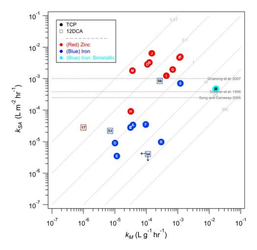
Figure 13. Mass-normalized rate constants ( $k_{\rm M}$ ) and the corresponding surface-area normalized rate constants ( $k_{\rm SA}$ ) for reduction of TCP and related chlorinated aliphatics by Zn<sup>0</sup> and Fe<sup>0</sup>. Diagonal lines are contours for representative values of  $\rho_{\rm a}$  (m<sup>2</sup> g<sup>-1</sup>). Horizontal lines represent  $k_{\rm SA}$ 's for TCP and Fe<sup>0</sup> estimated from QSARs previously published in the noted sources.
