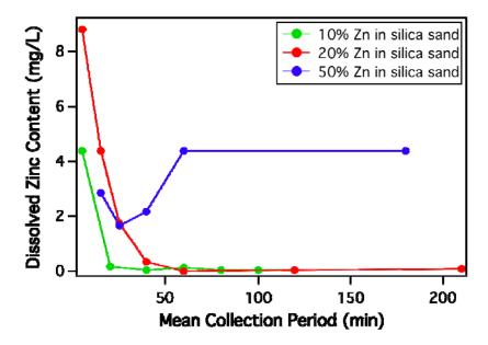
Figure 40. Effect of mass concentration of ZVZ in sand on effluent concentrations of Zn<sup>2+</sup> over time.
