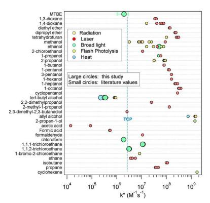
Figure 20. Comparison of all available second-order rate constants for reaction of sulfate radicals with environmentally relevant aliphatic organics. The large circles are values that we measured for another project. The color coding shows that the method of persulfate activation does not have any necessary effect on k".
