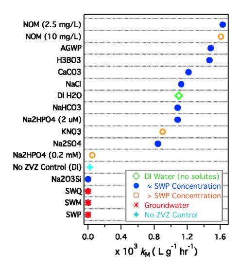
Figure 29.  $k_{\rm M}$  values obtained from observed values shown in Figure 28 for TCP degradation by Zn64 in DI water, site groundwaters P, Q, and M, and various artificial groundwaters prepared at or above the concentration reported for Site Water P (SWP).
