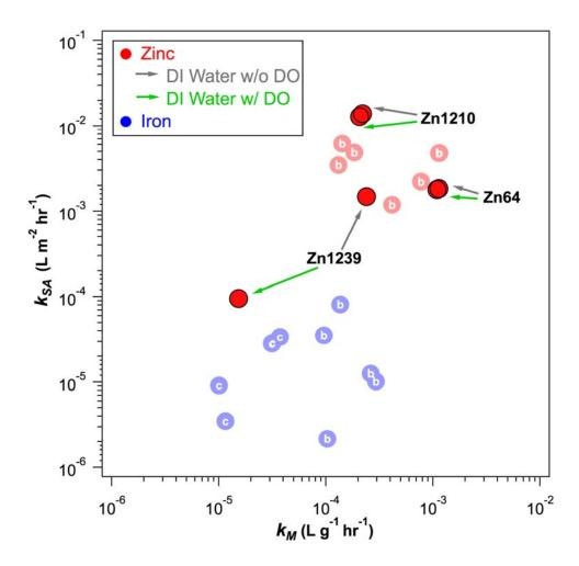
Figure 24. Comparison of TCP degradation kinetics by industrial-grade ZVZ materials to values gathered with reagent-grade ZVZ and various zero-valent iron (ZVI) materials as reported in (4). Kinetics were measured in DI water with and without dissolved oxygen. Kinetics in the presence of reagent- and industrial-grade ZVI (as reported in (4)) are shown for comparison.
