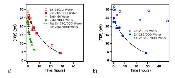
Figure 22. (**A**) Degradation of TCP by Zn64 and Zn1210 in DO/DI and DI water. (**B**) Degradation of TCP by Zn1239 in DO/DI and DI water. In both figures, solid symbols represent DO/DI data, with fit curves shown. Hollow symbols represent data from unsparged DI water batches. All batches contained an equal mass dose of ZVZ (250 g/L).
