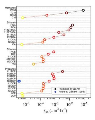
Figure 5. Rate constants ( $k_{SA}$ ) for degradation of chlorinated methanes, ethanes, ethenes, and propanes by Fe<sup>0</sup>. Yellow to black symbols represent predicted values calculated from QSARs described in (8). Blue symbols represent experimental data from (10).
