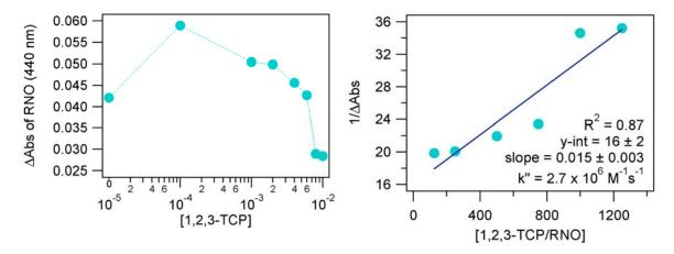
Figure 19. Preliminary competition kinetics for TCP degradation by activated persulfate. Light activation, pH = 9.
