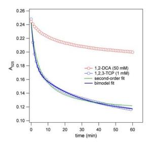
Figure 21. Disappearance of TCP and DCA in permanganate. (KMnO<sub>4</sub> = 0.1 mM, pH = 7.0, T =  $25^{\circ}$ C)
