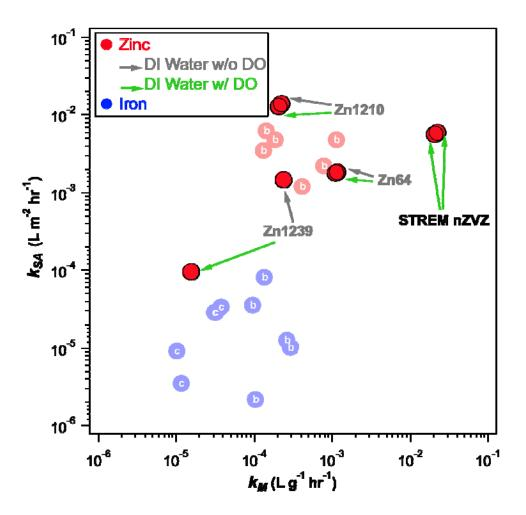
Figure 25. Comparison of nZVZ rates to rates gathered with industrial-grade ZVZ and to previously reported (4) ZVZ and ZVI rates.
