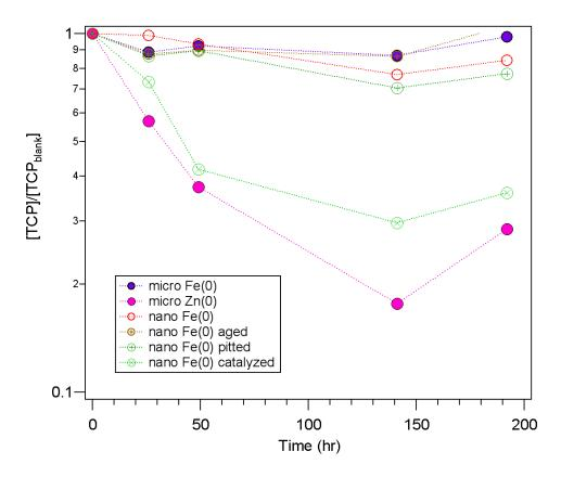
Figure 6. Results of batch experiments done with TCP and a variety of heterogeneous reductant systems. The micro Fe<sup>0</sup> was Fisher electrolytic and the nano Fe<sup>0</sup> was RNIP from Toda. The Zn<sup>0</sup> results are discussed in more detail below. The "Fe<sup>0</sup> catalyzed" experiments where done with RNIP that was modified with covalently bound iron-phthalocynanine.
