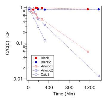
Figure 18. Pseudo first-order disappearance kinetics of TCP in unbuffered, heat activated, persulfate. Fitting these data gives  $k_{obs} = 0.15$ -  $0.19 \, \text{hr}^{-1}$  and  $t_{1/2} = 4 \, \text{hr}$  for anoxic conditions, and  $k_{obs} = 0.39 \, \text{hr}^{-1}$  and  $t_{1/2} = 1.8 \, \text{hr}$  for oxic conditions.
