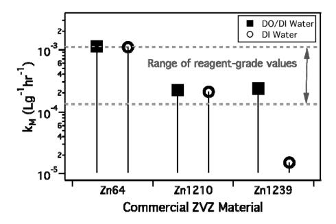
Figure 23. Mass normalized rate constants ( $k_{\rm M}$ ) for TCP degradation by three commercial ZVZ materials in DI water with and without dissolved oxygen. Gray dashed lines represent the range of  $k_{\rm M}$  values reported previously using reagent-grade ZVZ (4).
