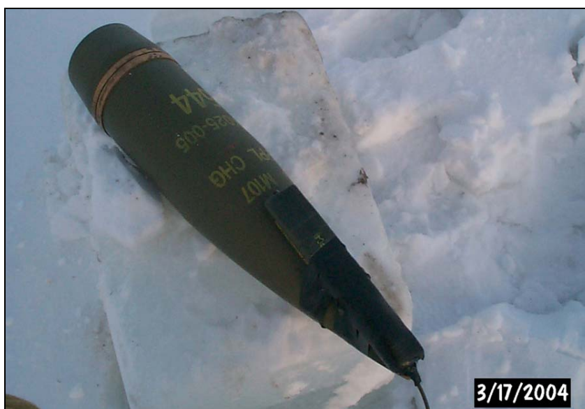
Figure 3. Detonation setup for 155-mm implementation tests.
