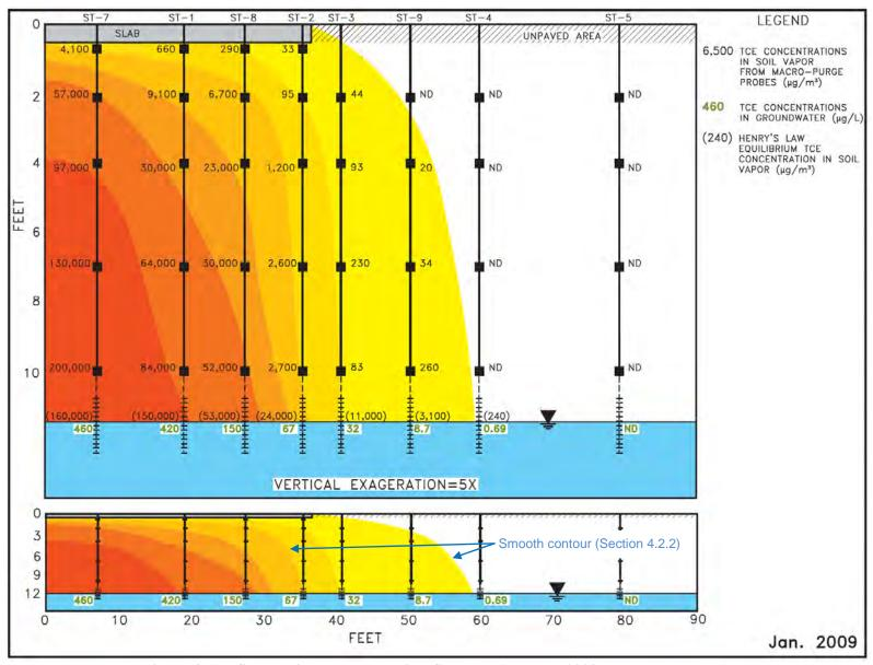
Figure 4-6 Schematic Isoconcentration Contours (January 2009 macro-purge data)
