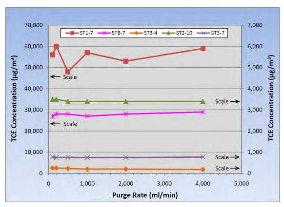
Figure 4-12 Linear Plot of Purge Rate Experiment Data
