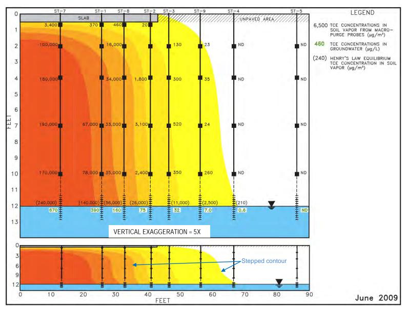
Figure 4-9 Schematic Isoconcentration Contours (June 2009 macro-purge data)
