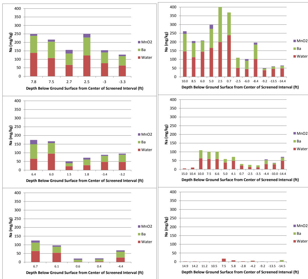
Figure 11. Sodium as water-extractable, Ba-extractable, and associated with MnO 2 solids structure for the test plot cores collected immediately post-treatment (left) and 1-year post-treatment (right) with respect to depth (relative to the center point of the screened interval).
