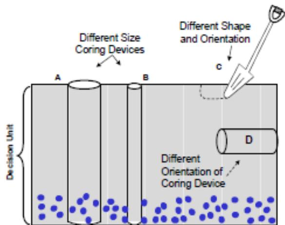
**Figure 2-14. Increment DE and EE from sampling device selection.**
