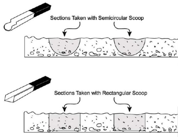
**Figure 2-12. Illustration of the effects of sampling device design on particle sizes in a sample.** *Source:* Gerlach and Nocerino 2003.
