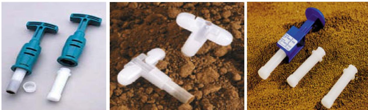
**Figure 5-12. Examples of coring devices for VOC soil increment collection.** Core N' One™ tool (left), Terra Core Sampler (center), and Easy Draw Syringe® and PowerStop Handle® (right).
