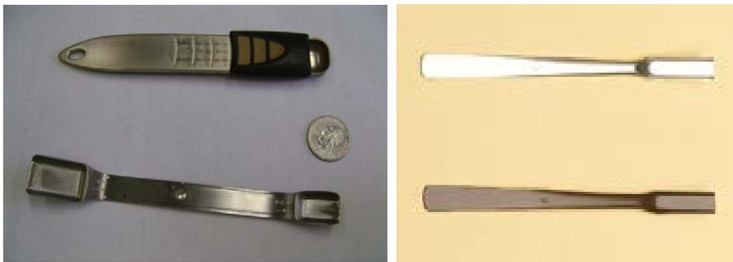
**Figure 5-9. Examples of rectangular and flat-bottom sampling tools.**
