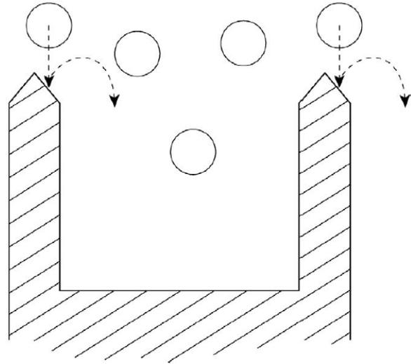
**Figure 2-13. Vertical view of a sampling device that minimizes EE.**
