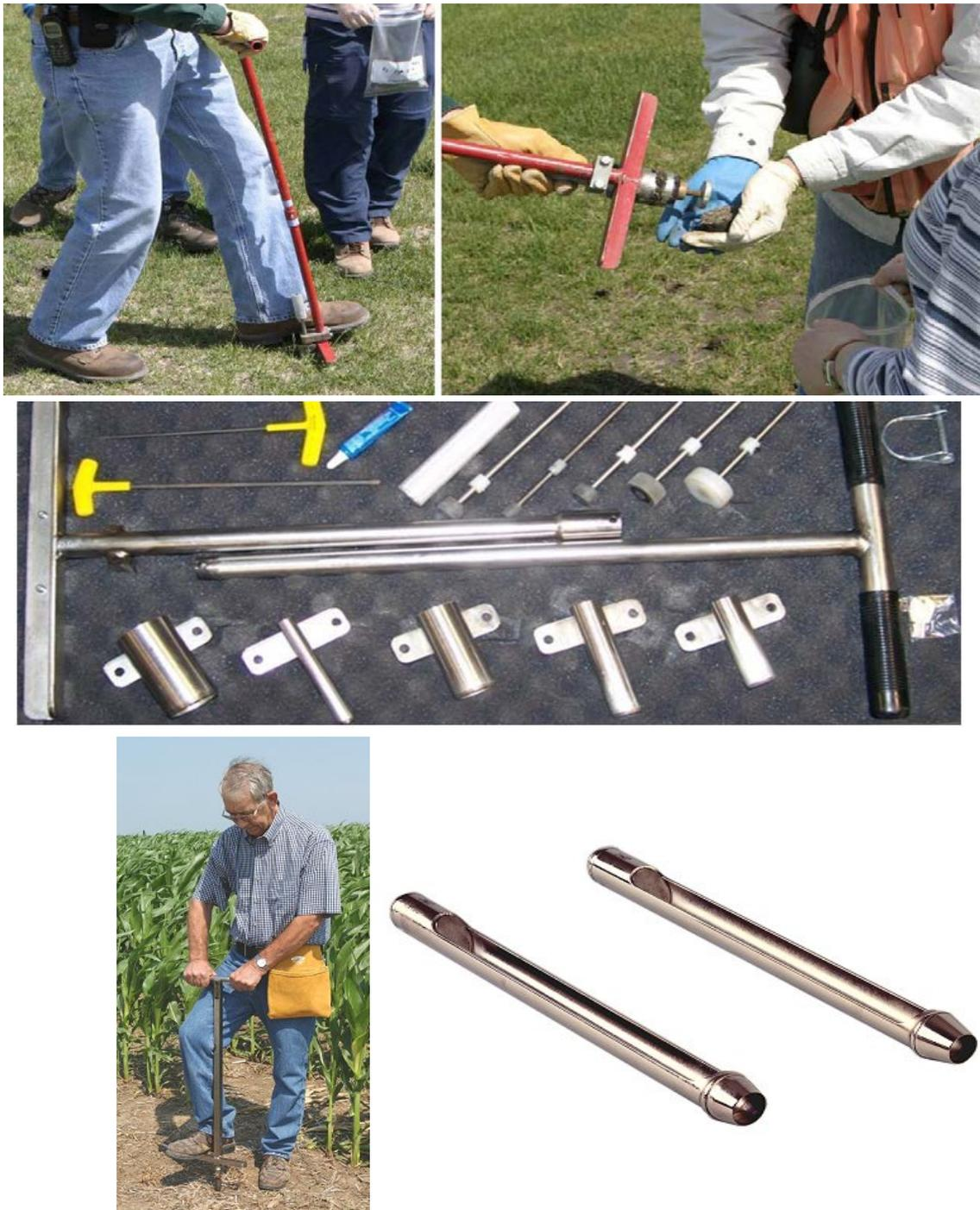
**Figure 5-2a. Examples of coring devices for nonvolatile soil increment collection. Top to bottom: Multi-Incremental Sampling Tool (MIST™), EVC Incremental Sampler, JMC Backsaver Handle, and Soil Tube.**
