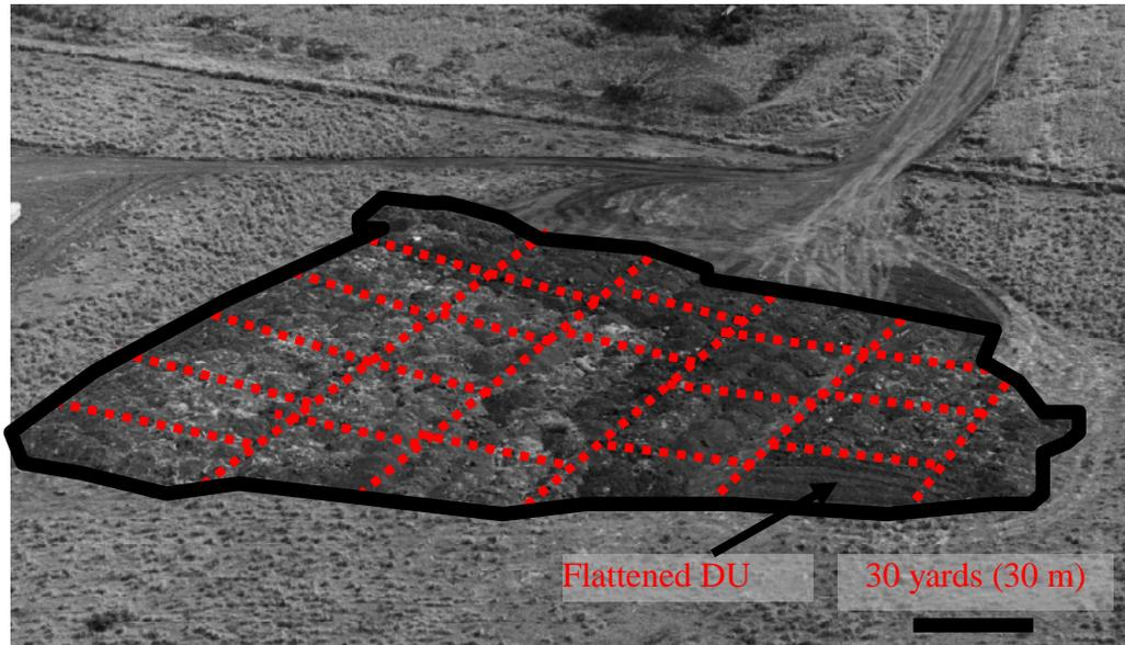
**Figure 3-10. Example of stockpile DUs.**
