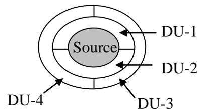
**Figure 3-6. Designation of perimeter DUs around a source area DU.**
