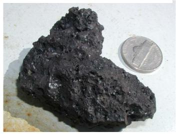
Close-up of Solidified Coal Tar, 5/05 Treated tar was dry, black and brittle (much like asphalt) 13
