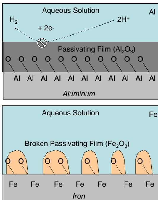
**Figure A9. Formation of passivation layers during the corrosion of iron (Fe) and aluminum (Al).** The passivation layer on Al is complete because the Al oxide forms a compatible passivating film. As drawn, the passivation occurs by blocking the cathodic reaction; however, anodic passivation is also possible. In contrast, the Fe oxide film is not compatible and forms oxides that are ineffective at blocking the surface.
