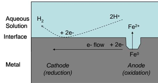
**Figure A3. Corrosion of iron in an aqueous solution of HCl. The anodic reaction generates the dissolved metal and electrons, which are transferred to the cathode, where they are used to reduce protons in solution. The extent of proton transfer is equal to the electron flow, a condition required to maintain charge neutrality.**
