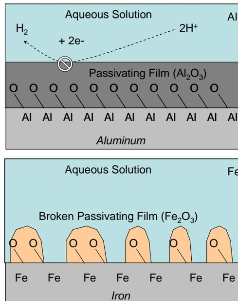
**Figure 12. Formation of passivation layers during the corrosion of aluminum (Al) and iron (Fe).** The passivation layer on Al is complete as the Al oxide forms a compatible passivating film. As drawn, the passivation occurs by blocking the cathodic reaction; however, anodic passivation is also possible. In contrast, the Fe oxide film is not compatible and forms oxides that are ineffective at blocking the surface.
