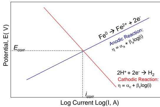
**Figure A5. Activation polarization curves for both anodic and cathodic reactions of Fe corrosion in dilute acid. The point at which the currents are equal defines the corrosion potential and current for the system. The curve with the steepest slope ultimately controls the corrosion potential as small changes in its slope or position significantly change the corrosion current.**
