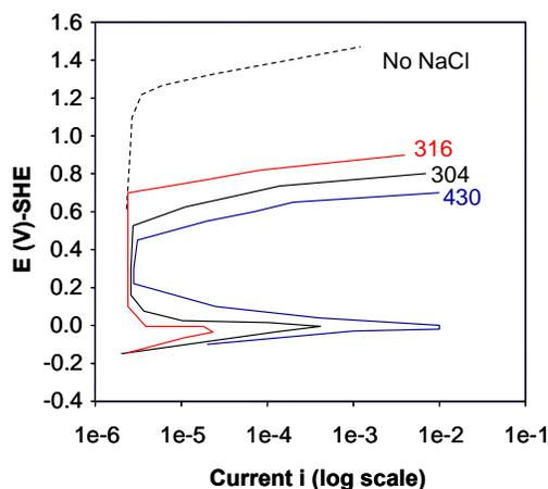
**Figure A12. Effect of alloy composition on steel corrosion. Anodic polarization for Stainless Steels of various composition (316, 304, and 430) in 0.05 M H<sub>2</sub>SO<sub>4</sub> and 0.01 M NaCl. The steel alloy changes the corrosion in the active region, and influences the potential of the transpassive region, where pitting occurs. The dotted line shows the anodic polarization curve for all steels in the absence of NaCl. Based on data from Talbot and Talbot (1998).**
