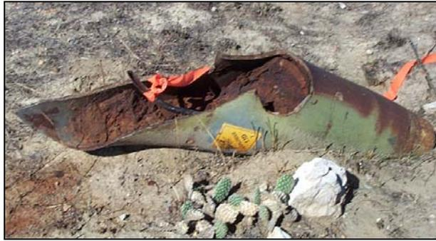
**Figure 18. Low-order detonation of a 500-lb bomb.**
