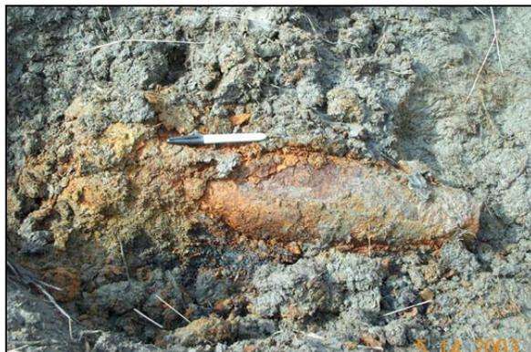
**Figure 13. Corroded 155-mm howitzer round found in wetland sediments at Eagle River Flats, Alaska.**
