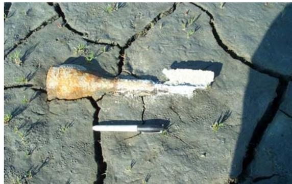
**Figure 5. Corrosion of an aluminum fin on a 81-mm mortar found at Eagle River Flats, Alaska.**
