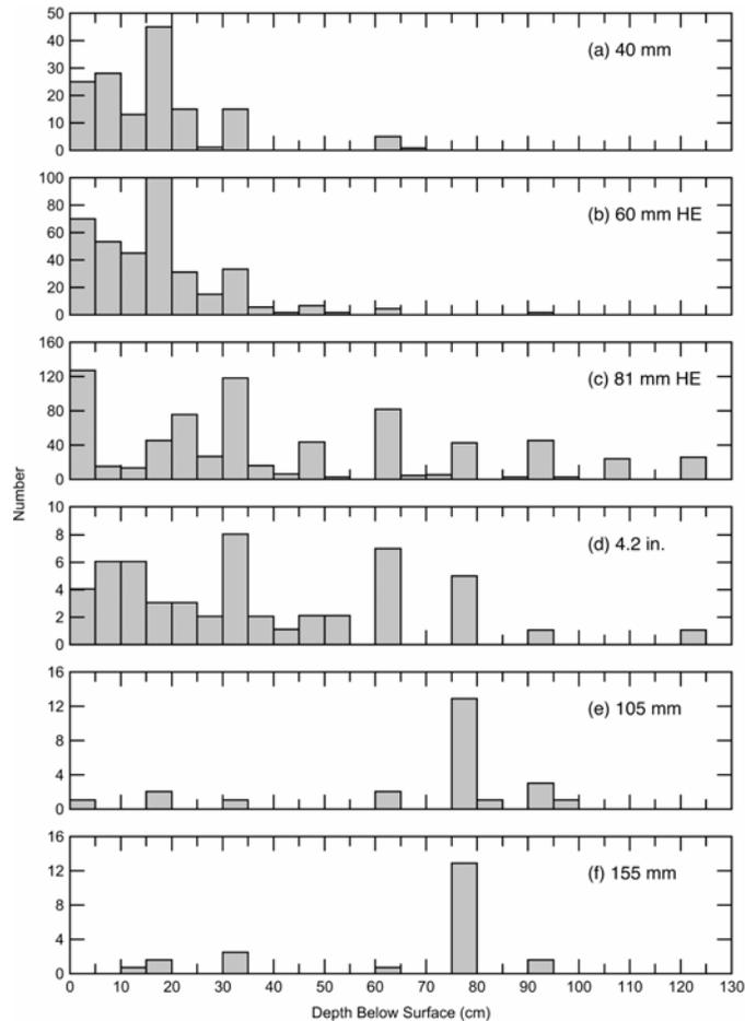
**Figure 7. UXO as a function of depth.**
