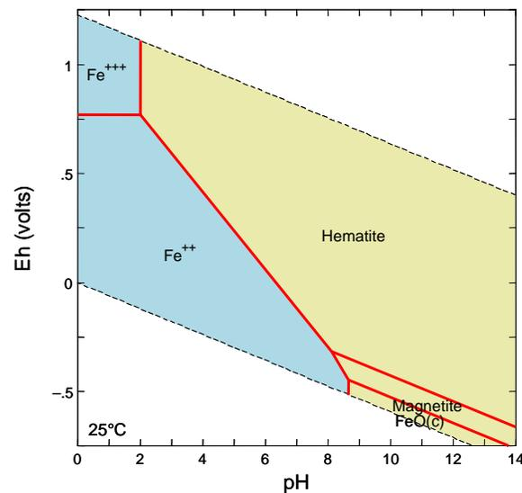
**Figure 9. Fe phase diagram for Fe-O<sub>2</sub> system at 25°C.** The diagram is derived using a dissolved Fe concentration of 1  $\mu\text{M}$ . Darker colored phases are aqueous, while lighter phases are solids. The diagonal dotted lines show boundaries for the stability of water; the vertical dotted line shows the change in carbonate speciation. Hematite is  $\alpha\text{-Fe}_2\text{O}_3(\text{s})$ .
