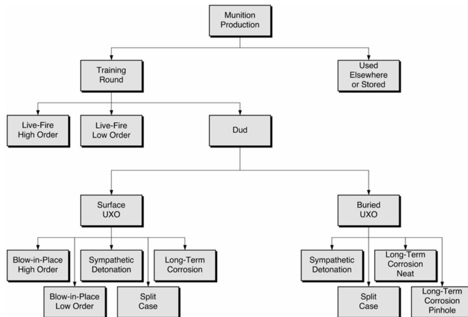
Figure 6. Possible fates of a fired munition.
