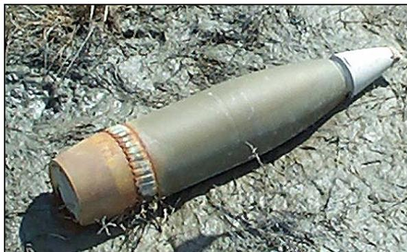
**Figure 4. Corrosion of a copper rotating band on a 155-mm round found at Eagle River Flats, Alaska.**
