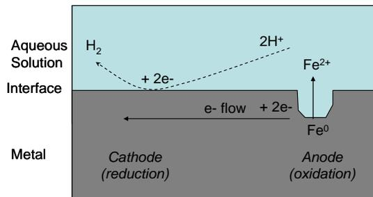
**Figure 11.** Corrosion of iron in an aqueous solution of HCl. The anodic reaction generates the dissolved metal and electrons, which are transferred to the cathode, where they are used to reduce protons in solution. The extent of proton transfer is equal to the electron flow, a condition required to maintain charge neutrality.
