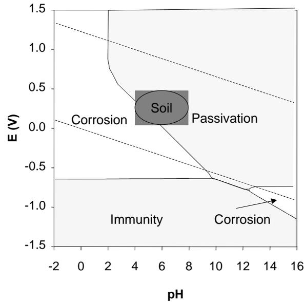
**Figure A8. Domains in which passivation of iron can occur. Note that these domains are very similar to those in which solid phases are formed. Immunity occurs in E-pH domains where there is no thermodynamic driving force for corrosion. The dotted lines indicate the stability zone of water and the shaded oval is the domain in E-pH space that is most prevalent in soils.**
