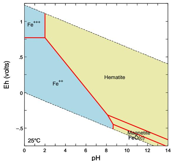
**Figure A1. Fe phase diagram for Fe-O<sub>2</sub> system at 25°C.** The diagram is derived using a dissolved Fe concentration of 1 μM. Dark shaded phases are aqueous, while lighter phases are solids. The diagonal dotted lines show boundaries for the stability of water; the vertical dotted line shows the change in carbonate speciation. Hematite is α-Fe<sub>2</sub>O<sub>3</sub> (s).
