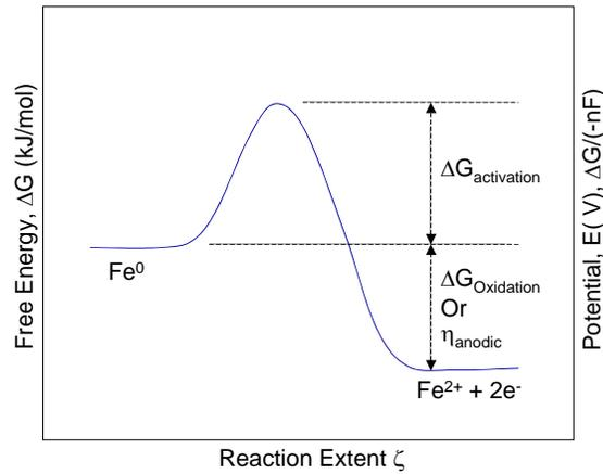
**Figure A4. Coordinate diagram for an activation controlled (chemically controlled) reaction. The reaction extent describes the conversion of reactants at the left, to products at the right. The reaction rate is proportional to current, and depends on the fraction of the population that has energy in excess of the free energy of activation (which is determined by Boltzmann's distribution).**
