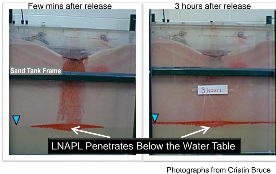
This sand tank experiment shows the release of an LNAPL dyed red. The second image shows that the LNAPL distributes above and below the water table, as expected.
