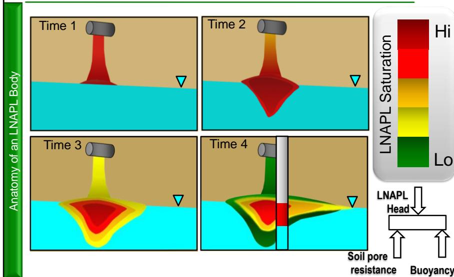
Shows evolution of an LNAPL body over time, starting with the initial release.
