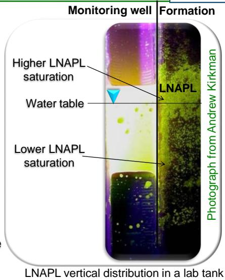
The key message here is that LNAPL doesn't float like a pancake on top of the water table, it penetrates below the water table in a variable saturation profile. This varying saturation arises because the LNAPL and water occupy the same pore space.
