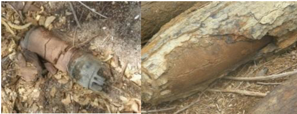
Figure 5. Explosive fill exposed by corrosion of UXO casings.
