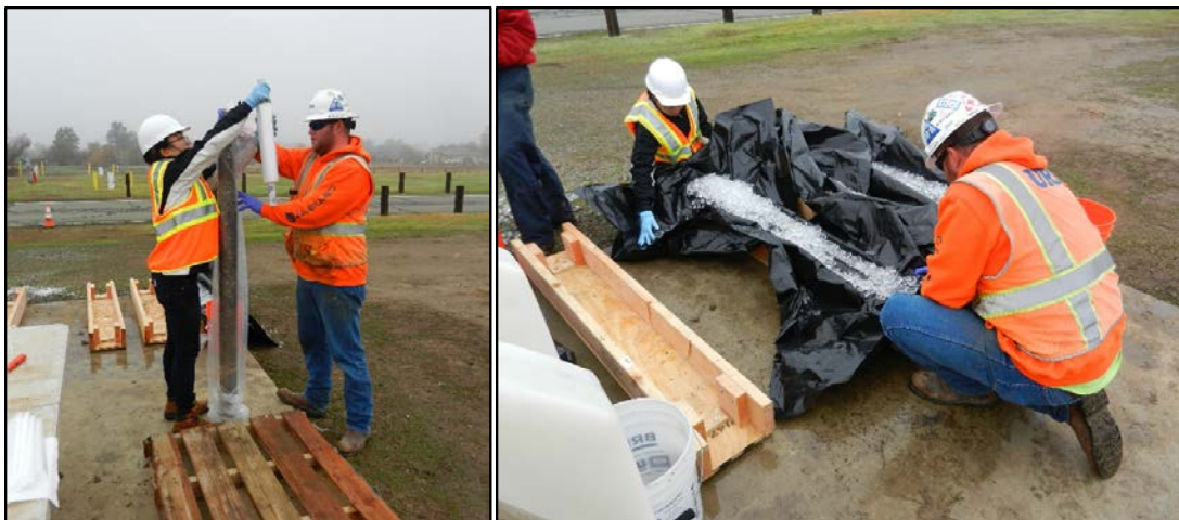
Figure 5.7.24. Split Spoon Cool Down Procedure During Post-demonstration Soil Sampling.
