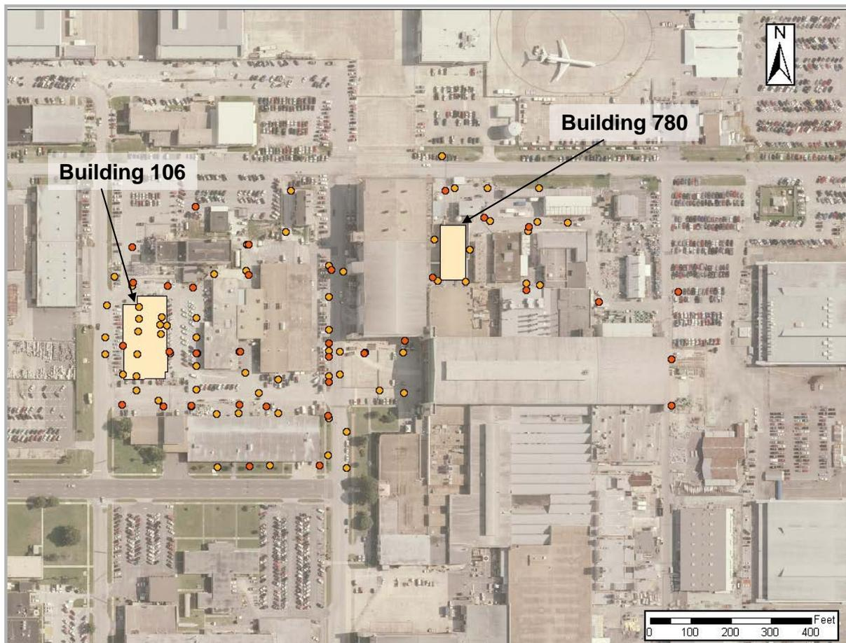
**Figure 4.2. Site Map of OU3 at NAS Jacksonville.** Figure shows only a portion of OU3, specifically the focus areas for the current project, including Building 106 and Building 780. Colored dots represent investigation points (primarily MIP and/or CPT) that were part of previous site characterization activities. (Modified from figure supplied by site manager)
