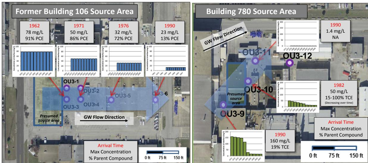
**Figure ES.1. Plume Arrival Times Based on Source History Modeling Results at Former Building 106 Source Area and Building 780 Source Area.** Dates reflect plumes arrival, concentrations reflect total chlorinated ethenes in the transmissive zone starting at that date, and percentages reflect contribution of parent compound (PCE or TCE) to total chlorinated ethene concentration.
