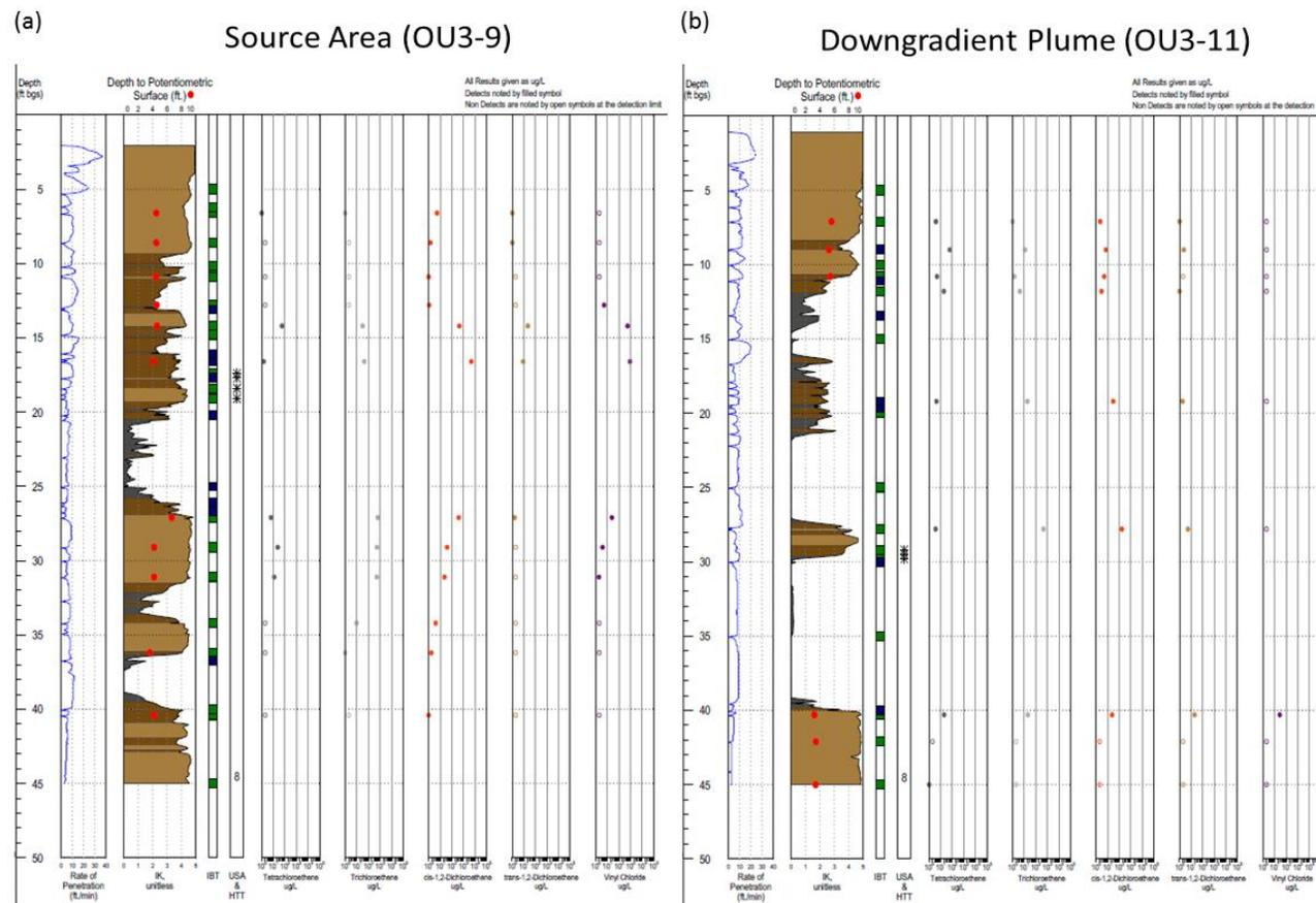
**Figure 5.12. Example of Waterloo APS™ Results at Building 780 Source Area:** (a) near source area, and (b) downgradient plume area showing the  $I_k$ , groundwater VOC concentrations, along with other complementary data collected including drive rate and potentiometric surface.
