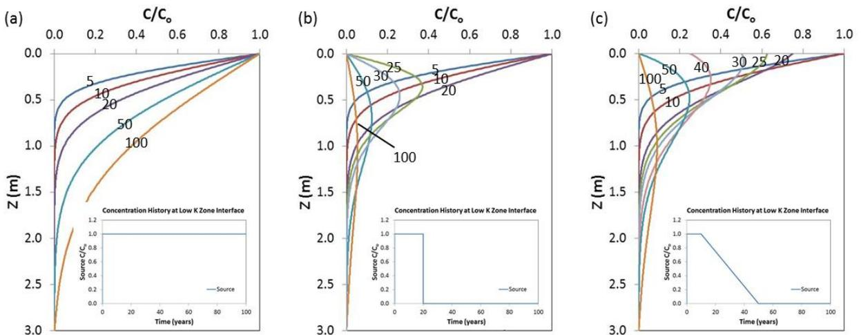
**Figure 2.1.** Low-k zone profiles for different historical interface concentration conditions: (a) constant concentrations, (b) constant concentrations for 20 years followed by complete removal of source, and (c) constant concentrations for 10 years followed by linearly declining concentrations with source depleted by 50 years.
