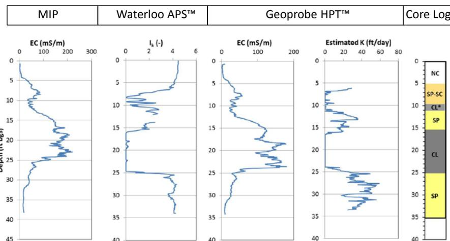
**Figure 5.13.** Stratigraphic Data Collected by Various Screening-Level Methods at Former Building 106 Source Area: (c) Location OU3-4; (d) Location OU3-5. Panels from left to right show data from MIP; Waterloo<sup>APS™</sup>; (c) Geoprobe HPT, and Soil Coring.
