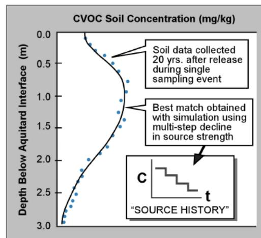
The Source History Tool generated by this project (see below for screenshot example) is a simple spreadsheet-based model that follows this approach to obtain a source history estimate that best represents the soil concentration profile. It also uses a vertical advection term and a first-order decay term to understand the potential impacts of these processes on contaminant fate and transport in addition to diffusion and sorption.
