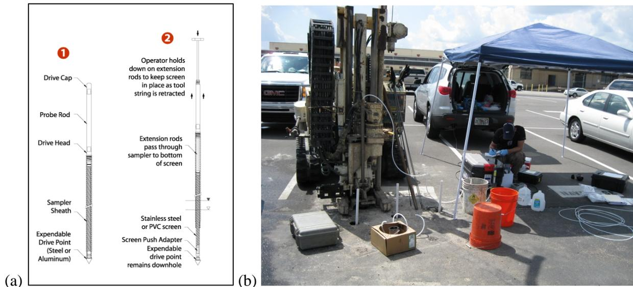
**Figure 5.8. Multi-Level Groundwater Sampling:** (a) Schematic of Geoprobe SP16 sampler operation (from <http://geoprobe.com/sp16-groundwater-sampler>); (b) Groundwater sampling during the ESTCP ER-201032 field demonstration, using Geoprobe SP16 system (via the direct-push rig) and temporary piezometers (installed in small diameter boreholes in foreground).
