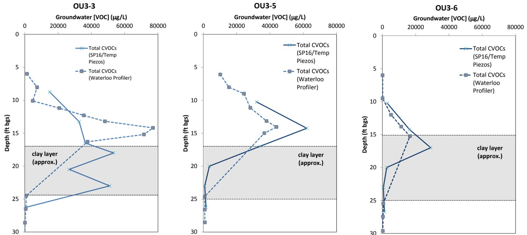
**Figure 5.16. Groundwater Total CVOC Concentrations from Former Building 106 Source Area Locations.** Locations from left to right represent plume flowpath from near source (OU3-3) to downgradient plume (OU3-6). Data were collected using either Geoprobe SP16/Temporary Piezometers or Waterloo<sup>APS™</sup>.
