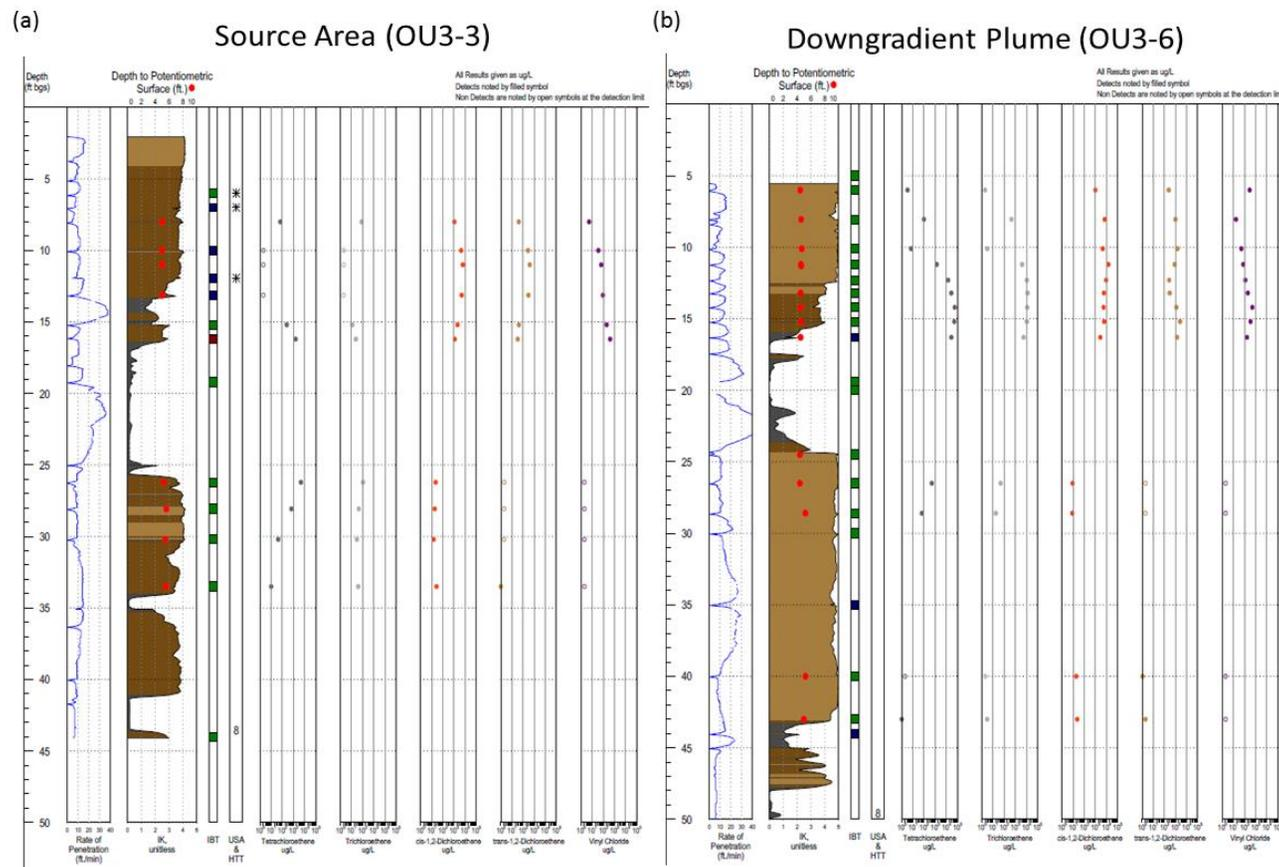
**Figure 5.11. Example of Waterloo APS™ Results at Two Locations at Former Building 106 Source Area: (a) near source area, and (b) downgradient plume area showing the I<sub>k</sub>, groundwater VOC concentrations, along with other complementary data collected including drive rate and potentiometric surface.**
