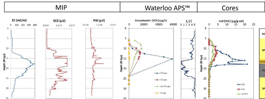
**Figure 5.18. Composite Plot of Characterization Data Collected at Former Building 106 Source Area:** (a) Location OU3-3; (b) Location OU3-4. Shown from left to right are results from MIP, Waterloo<sup>APS™</sup> (groundwater VOC concentrations and  $I_k$  data, and soil cores (soil VOC concentrations and geologic log). EC = electrical conductivity; ECD = electron capture detector; PID = photoionization detector; VOC = volatile organic compound;  $I_k$  = index of hydraulic conductivity.
