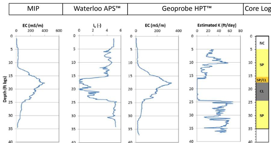
**Figure 5.13.** Stratigraphic Data Collected by Various Screening-Level Methods at Former Building 106 Source Area: (a) Location OU3-3; (b) Location OU3-4. Panels from left to right show data from MIP; Waterloo<sup>APS™</sup>; (c) Geoprobe HPT, and Soil Coring.
