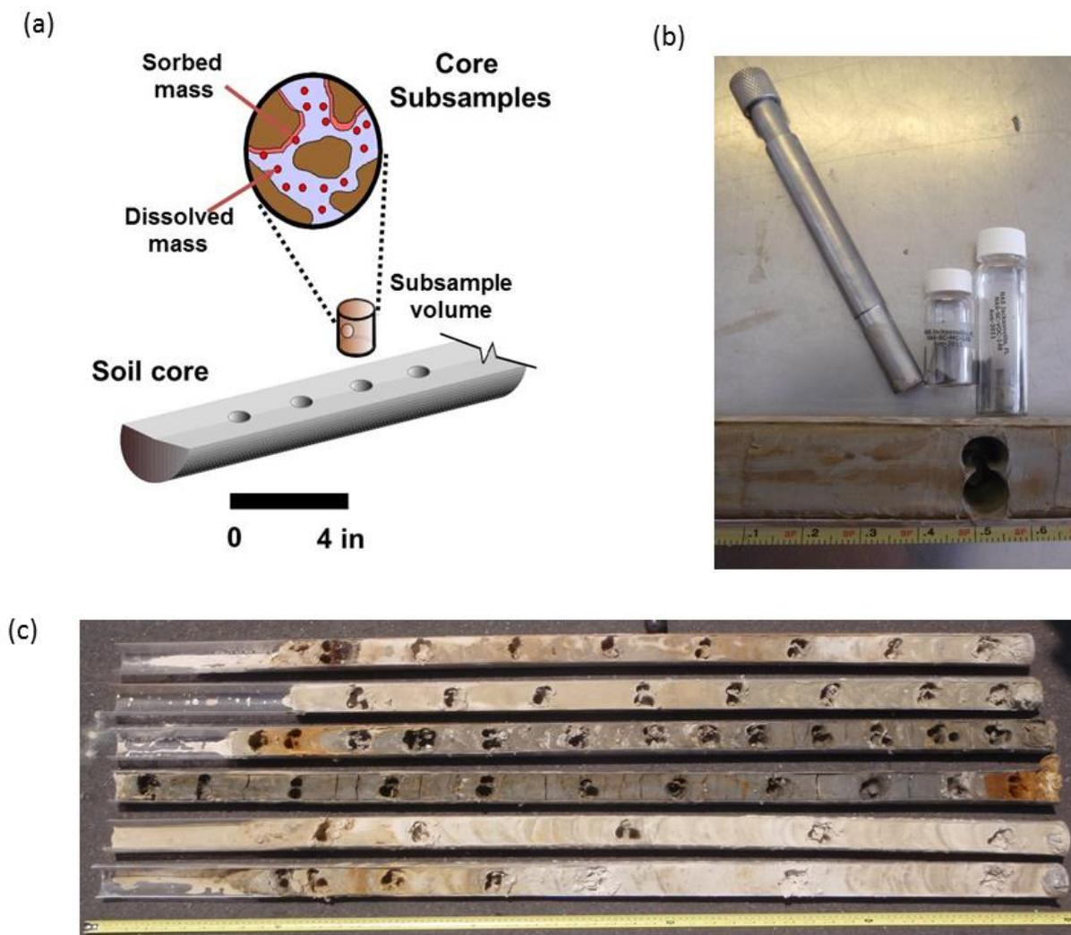
**Figure 5.7. High-Resolution Soil Sub-Sampling:** (a) schematic, (b) stainless steel subsampler and samples from one depth (one preserved in methanol for VOCs, one for moisture content), and (c) example of subsampled cores from OU3-4 (collected from 5-35 ft bgs).
