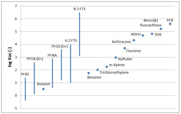
Figure 1. Partition coefficients between organic carbon and water (Koc) for a number of different PFCs as well as a number of common soil- and groundwater contaminants. Several of these PFSc are common at fire fighting sites where fire fighting foam has been used. Data for PFCs is taken from Gellrich and Knepper (2012) except 6:2 FTS and 8:2 FTS where values have been obtained using the models EPISUITE and ACD/Labs. Note logarithmic scale.
