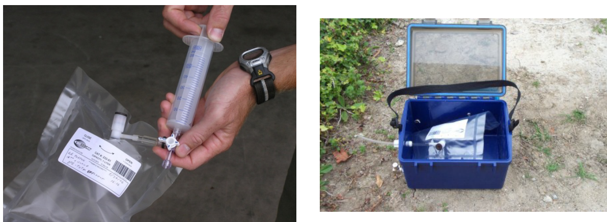
Figure G-15. (a) Filling a gastight bag using a syringe and three-way Luer valve. Top of the valve is connected to the probe tubing. (b) A vacuum chamber (sometimes called a lung-box) to inflate gastight bags.
