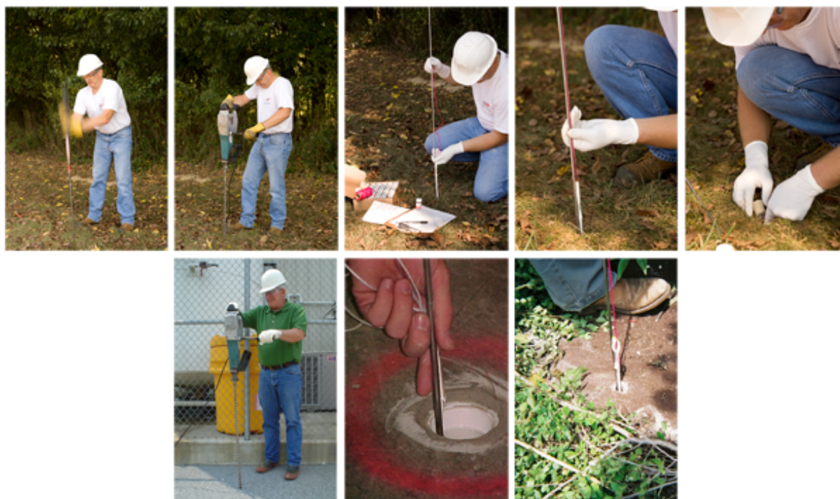
Figure G-4. Passive soil vapor sampler installation. Top: Exterior soil vapor sampling using slide hammer and rotary hammer drill, insertion of a passive soil gas sampler, and sealing the hole. Bottom: Subslab soil vapor sampling.
