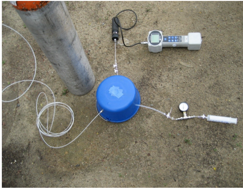
Figure G-13. Gas shroud over Vapor Probe Surface Completion. System consists of shroud (blue bucket), helium cylinder, field helium detector and syringe with vacuum gauge for purging.
