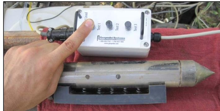
**Figure 8: As part of the field QA testing the EC probe is setup in the test jig (bottom) and the EC test load (top) is used to verify the performance of the EC array before each log is run. The QA results are saved in the information file (Appendix II).**
