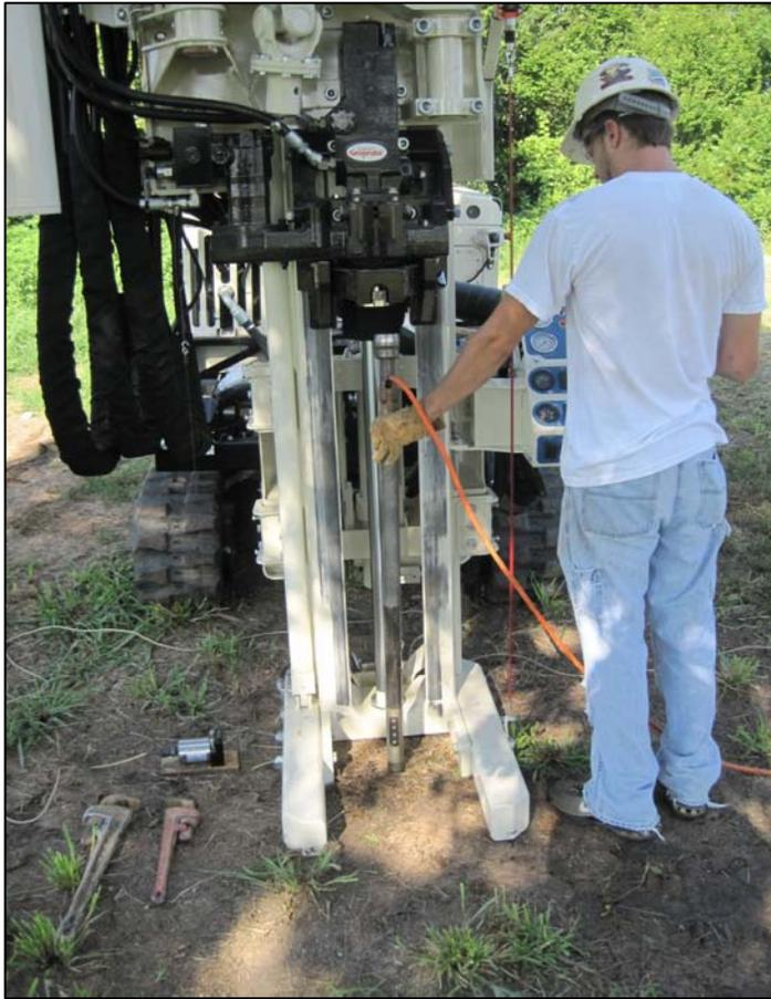
**Figure 2: Operator setting up HPT Probe for advancement into the subsurface with a Geoprobe® 7822 machine. The HPT probe is advanced at 2cm/sec using the system hydraulics and probe hammer when required. Logs to a depth of approximately 60ft (20m) are usually completed in about one hour.**
