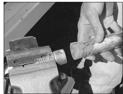
Figure 4.26. Move free end of liner back-and-forth to split liner and free it from the liner drive head.
