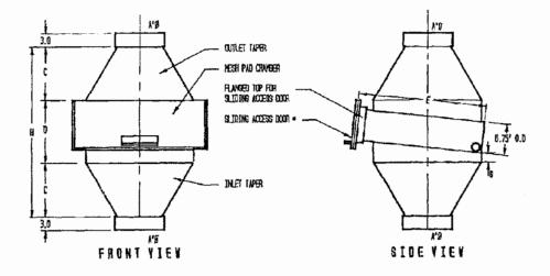
Figure 5: Vertical, In-Line Mesh pad Mist Eliminator (Source: KCH Services, Inc.)
