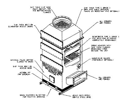
Figure 6: Vertical Mesh pad System (Source: Midwest Air Products Co. Inc.)
