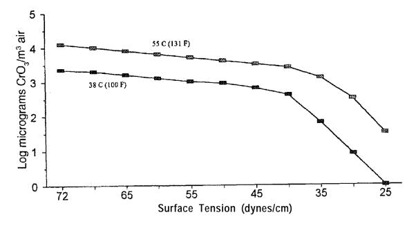
Figure 13 : Surface tension vs. chromic acid emissions (USEPA, 1993).
