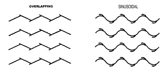
Figure 2: Blade Configurations Used in Chevron Mist Eliminators
