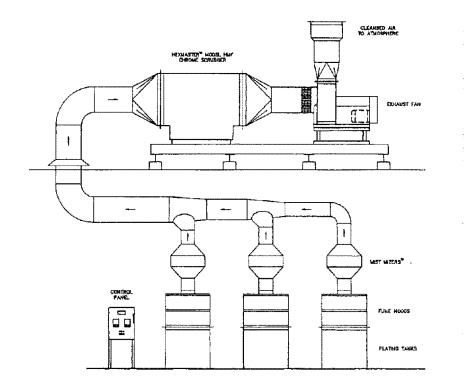
Figure 10: Combination In-Line and End-of-Line Mesh pad Devices (Source: Met-Pro Corporation, Dual1 Div.)
