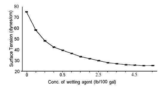
Figure 12: Wetting agent concentration vs. surface tension (USEPA, 1993)
