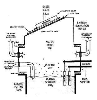
Figure 9: Encapsulating Tank Cover with Membrane and Evacuation Systems (Source: Responsible Alternatives Inc.)
