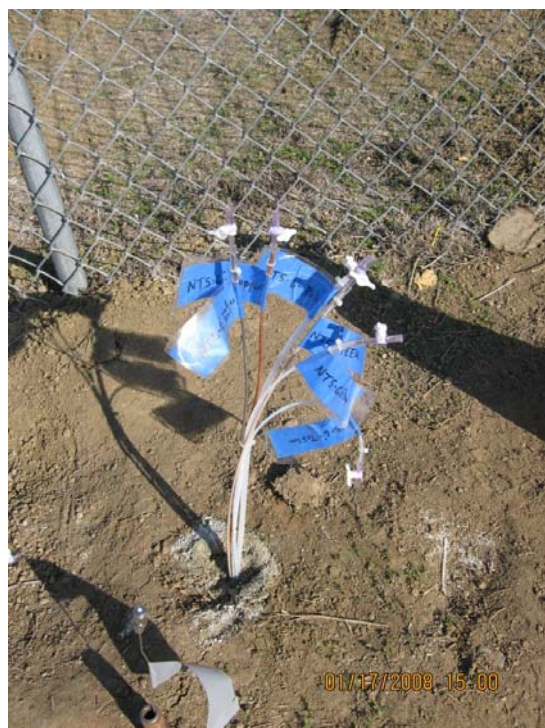
Photograph 9: EPA installing micro-purge soil gas probes.
