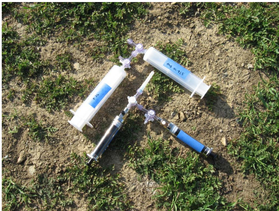
Photograph 16: Polypropylene (upper) and glass (lower) sampling syringes.
