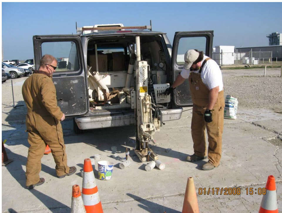
Photograph 8: EPA installing micro-purge soil gas probes.
