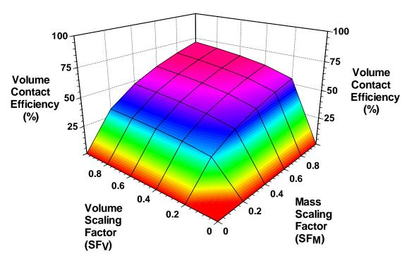
Figure 2.11. Effect of Volume Scaling Factor (SF<sub>V</sub>) and Mass Scaling Factor (SF<sub>M</sub>) on Volume Contact Efficiency ( $E_V$  for  $OR \ge 0.05 \ OR_M$ ) for a Moderately Heterogeneous Aquifer with Well Spacing Approximately Equal to Row Spacing.
