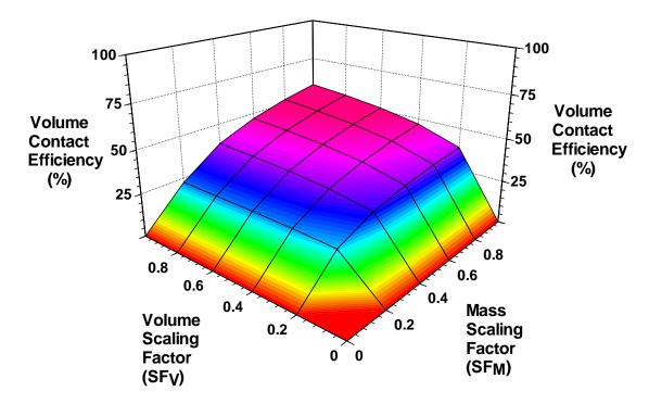
Figure 2.12 Effect of Volume Scaling Factor (SF<sub>V</sub>) and Mass Scaling Factor (SF<sub>M</sub>) on Volume Contact Efficiency ( $E_V$  for  $OR \ge 0.05$   $OR_M$ ) for a Moderately Heterogeneous Aquifer with Row Spacing Equal to Approximately Two Times Well Spacing.
