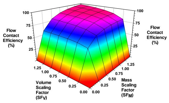
Figure 2.15. Effect of Volume Scaling Factor (SF<sub>V</sub>) and Mass Scaling Factor (SF<sub>M</sub>) on Flow Contact Efficiency (E<sub>F</sub> for  $OR \ge 0.05 \ OR_M$ ) for a Moderately Heterogeneous Aquifer (realization #2).
