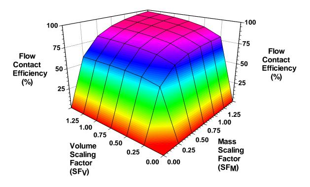
Figure 4.2. Contact Efficiency for Barrier Treatment.
