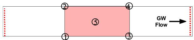
Figure 2.2. Model Domain for Base Case Condition – Area Treatment.
