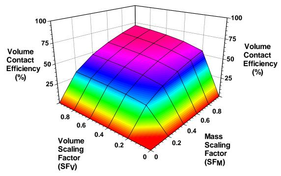
Figure 4.4. Contact Efficiency for Area Treatment when Row Spacing = Well Spacing.
