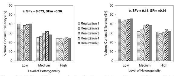
Figure 2.7. Effect of Heterogeneity Realization on Volume Contact Efficiency ( $E_V$ ) for Low, Moderate and High Heterogeneity Aquifers.
