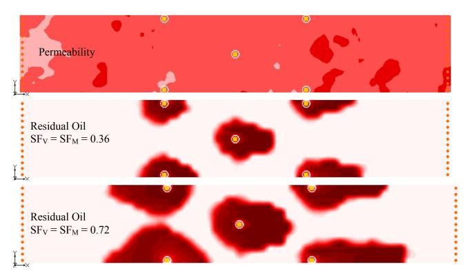
Figure 2.3. Simulated Horizontal Distribution of Hydraulic Conductivity and Residual Oil in Top Layer of Aquifer (see Figure 2.4) for Moderately Heterogeneous Aquifer (realization #2).
