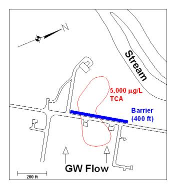
Figure A3.1. Map of the Maryland Site Showing Plume of Elevated TCA ( $\mu g/L$ ) in Red and Location of the Proposed Barrier in Blue.
