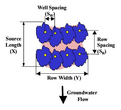
Figure 4.3. Emulsified Oil Area Treatment Design Schematic.
