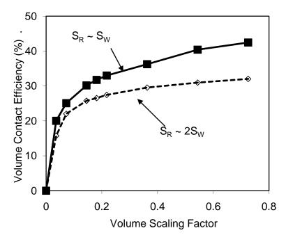
Figure 2.10. Effect of Row Spacing and Fluid Injection Volume on Volume Contact Efficiency ( $E_V$  for  $OR \ge 0.05$   $OR_M$ ) for a Moderately Heterogeneous Aquifer.
