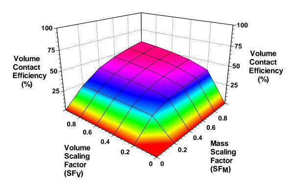
Figure 4.5. Contact Efficiency for Area Treatment when Row Spacing = 2 \* Well Spacing.
