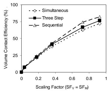
Figure 2.6. Effect of Injection Sequence and Scaling Factor on Volume Contact Efficiency ( $E_V$  for  $OR \ge 0.05$   $OR_m$ ) at 120 Days for a Moderately Heterogeneous Aquifer (permeability realization #2).
