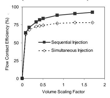
Figure 2.14. Effect of Injection Sequence and Fluid Injection Volume on Flow Contact Efficiency ( $E_F$  for  $OR \ge 0.05$   $OR_M$ ) at 120 days for a Moderately Heterogeneous Aquifer (realization #2, Mass Scaling Factor = 0.86).
