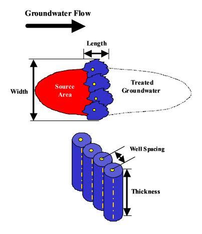
Figure 4.1. Emulsified Oil Barrier Design Schematic.
