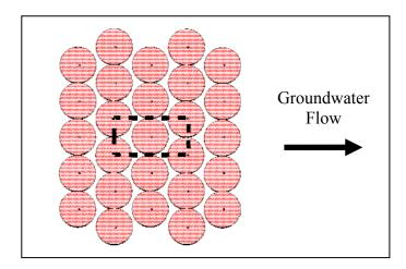
Figure 2.1. Hypothetical Injection Grid Showing Model Domain Subarea.
