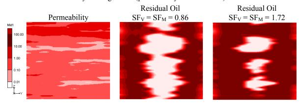
Figure 2.13. Simulated Distribution of Hydraulic Conductivity and Residual Oil in Cross-section Immediately Downgradient of Wells 1 and 2 for Moderately Heterogeneous Aquifer (realization #2).
