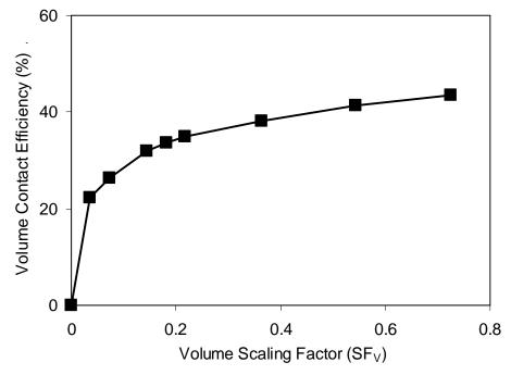
Figure 2.8. Effect of Volume Scaling Factor (SF<sub>V</sub>) on Volume Contact Efficiency (E<sub>V</sub> for C  $\geq$  0.05 OR<sub>M</sub>) for a Moderately Heterogeneous Aquifer at 120 days (Mass Scaling Factor = 0.36).
