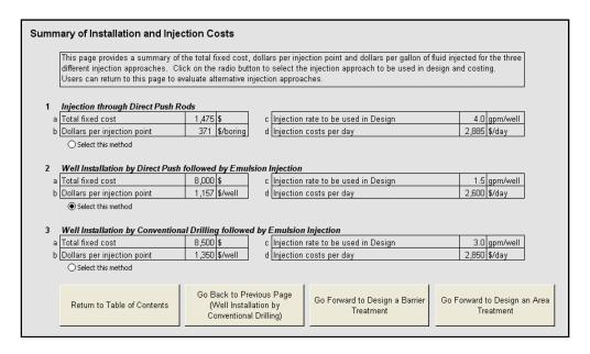
Figure A3.3. Summary of the Different Methods that Shows Which Items are Used in the Design.
