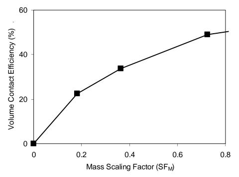
Figure 2.9. Effect of Mass Scaling Factor (SF<sub>M</sub>) on Volume Contact Efficiency ( $E_V$  for  $C \ge 0.05 \ OR_M$ ) for Sequential Injection of a Moderately Heterogeneous Aquifer at 120 Days.
