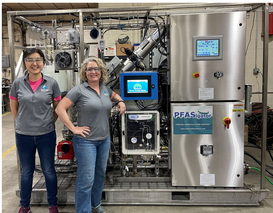
Figure E-3. Commercial-scale PFASigactor photo. The footprint of the equipment is 9' (Length) x 7' (Height) x 4' (Width). Co-founders of Enspered Solutions, Dr. Meng Wang (left) and Dr. Denise Kay (right) stand in front of the equipment.
