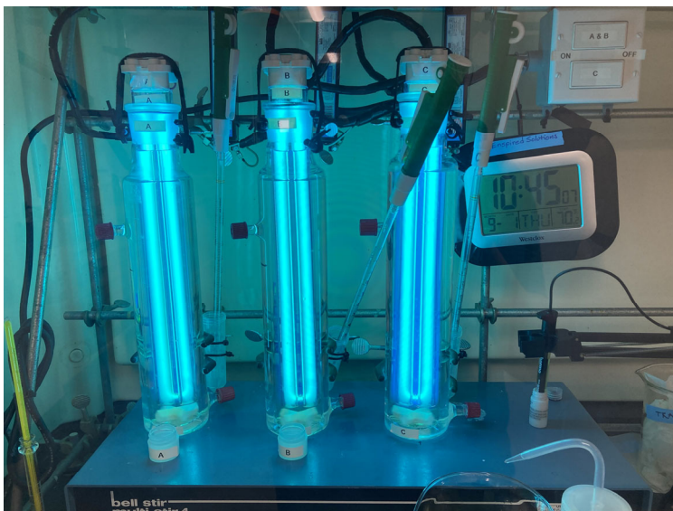
Figure 5-2. Benchtop test reactor set up for small scale treatability studies.
