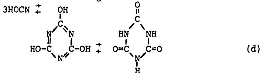
The cyanic acid is found in the reaction of RDX products with ozone after exposure to UV radiation only (experiment 3). Thus, it is attractive to consider that the major product from the UV radiation only is s-triazine (equation (e)). This product might be oxidized by ozone to cyanuric acid directly, and/or may undergo ozonolysis of the  $-\text{CH}=\text{N}-$  linkage (8) followed by decomposition to cyanic and fulminic acids:
