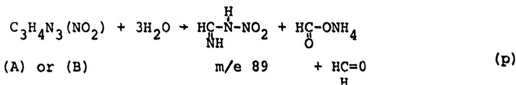
The two m/e 117 compounds (Figures 5 and 6) also form in the absence of ozone. The spectra of each indicate the presence of a nitro group (P - 46) and possibly, a formate linkage (HC=O, P - 29). Considering that P - 29 yields m/e 88 (m/e 89 minus one), one of the m/e 117 compounds may have the structure
