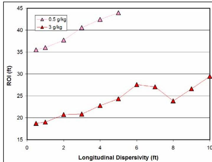
Figure A12-8: ROI Output vs. Longitudinal Dispersivity (half-reactor length).
