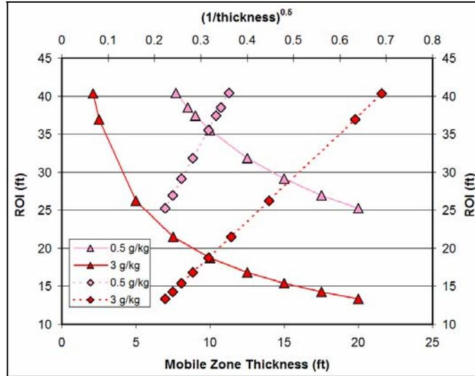
**Figure A12-6: ROI Output vs. Mobile Zone Thickness (triangle symbols and solid lines) and ROI Output vs. Normalized Mobile Zone Thickness (diamond symbols and dashed lines).**
