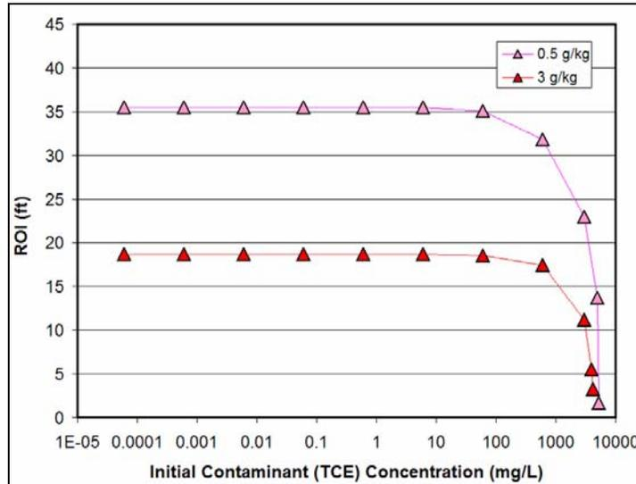
Figure A12-13: ROI Output vs. Initial Contaminant Concentration (note log scale of x-axis).
