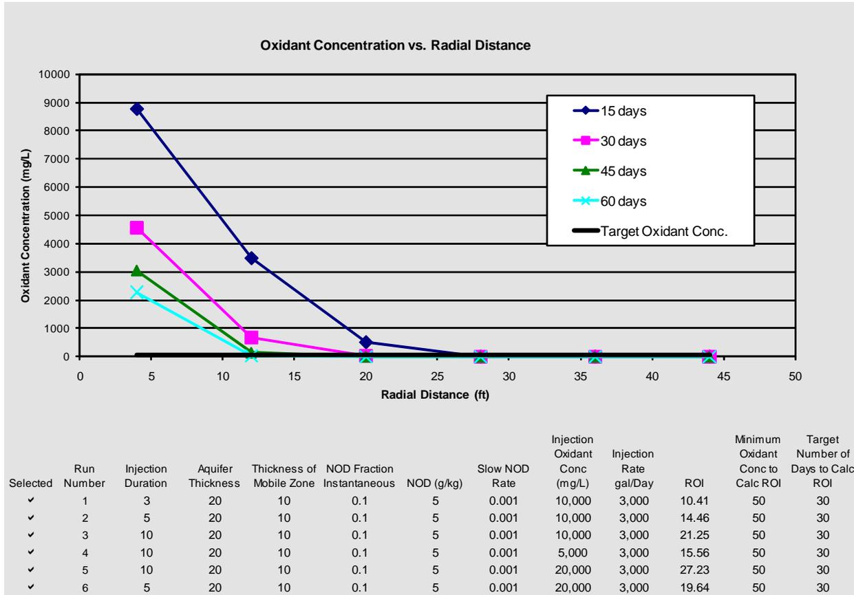
Figure A12-1: Typical Output from Permanganate Transport Model.
