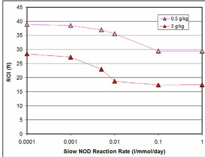
Figure A12-12: ROI Output vs. Slow NOD Reaction Rate (note log scale of x-axis).
