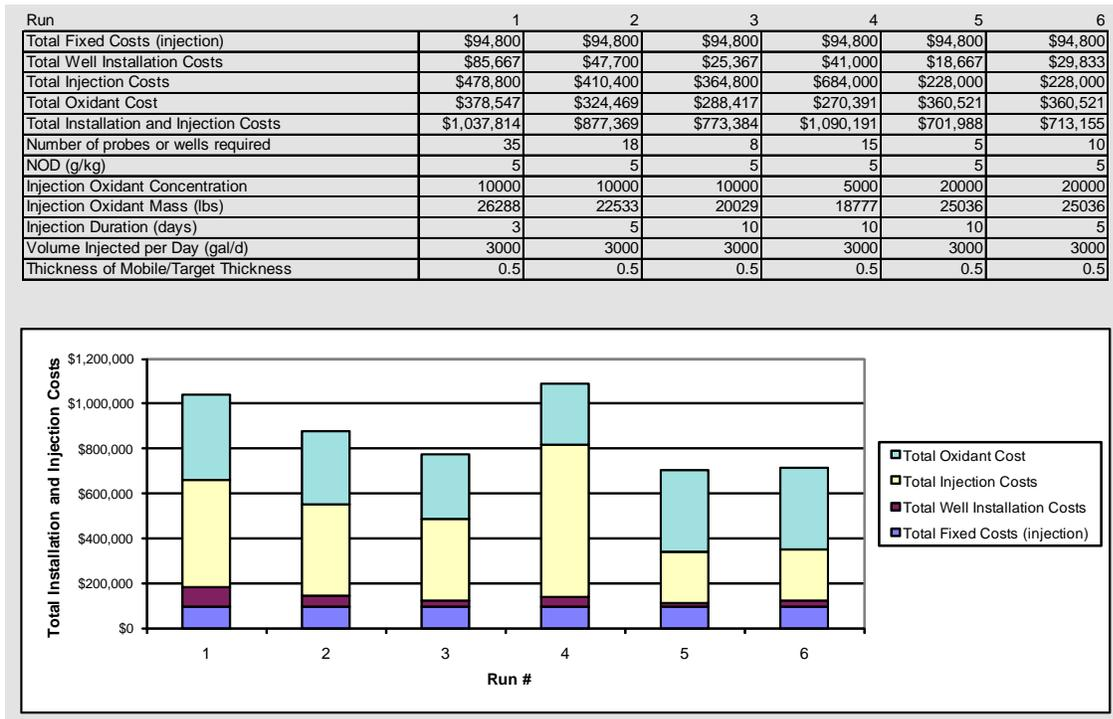
Figure A12-2. Typical Output from Injection Scenario Cost Comparison.
