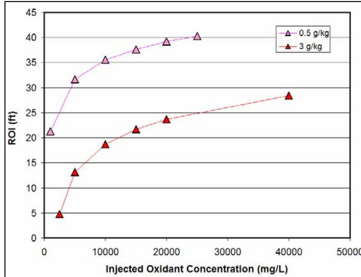
Figure A12-14: ROI Output vs. Injected Oxidant Concentration.
