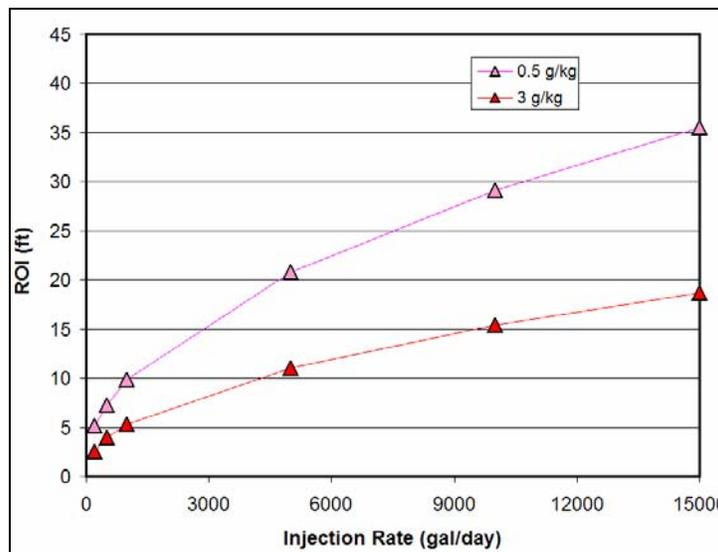
Figure A12-15: ROI Output vs. Injection Rate.
