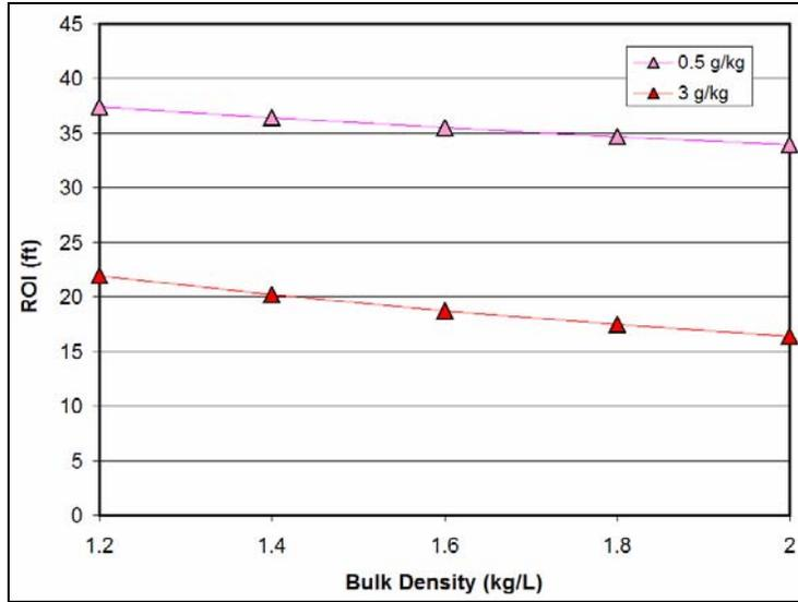
Figure A12-9: ROI Output vs. Bulk Density.
