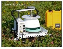
months) can be taken with the devise (LI-COR, 2014). The NSZD rate is calculated by correcting for the naturally occurring  $CO_2$  efflux using either the background  $CO_2$  efflux correction (Sihota et al., 2011) or the radio-isotope of carbon (<sup>14</sup>C; Sihota and Mayer, 2012).
