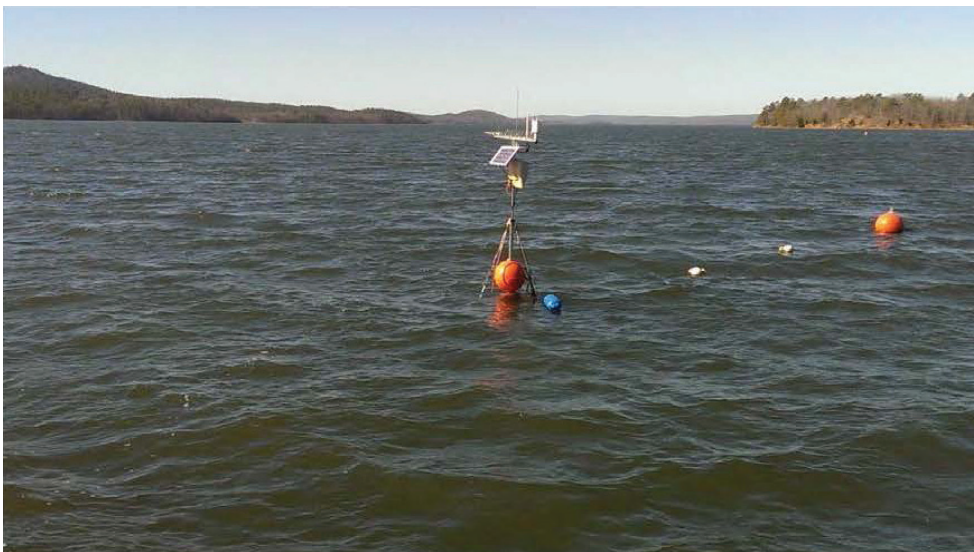
Figure 10–14. Buoyed continuous water-quality monitoring system on Lake Maumelle, Arkansas, station 072623995 (photograph by W.R. Green).
