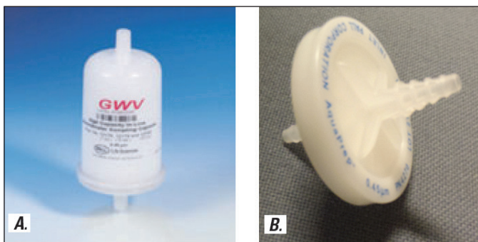
Figure 2–11. Disposable filtration devices: (A) GWV ® high-capacity capsule filter, 0.45- \mu m pore size, 700-cm 2 pleated Versapor ® filter membrane; and (B) Small-capacity AquaPrep ® disk filter, 0.45 \mu m, 19.6 cm 2 Versapor/Thermopor ® filter membrane. A, image courtesy of Pall Corporation; B, photograph by S.C. Skrobialowski, U.S. Geological Survey.
