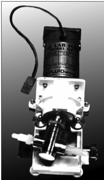
Figure 2–13. Valveless piston metering pump. Photograph by B.A. Bernard, U.S. Geological Survey.
