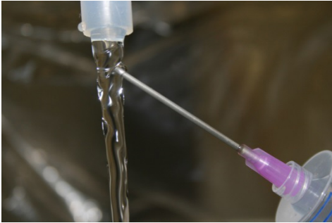
Figure 5.2.2.B-4. Use the bore needle to obtain groundwater for rinsing and conditioning the bore needle and syringe. (Photograph taken inside a sample-processing chamber by Michael Manning, U.S. Geological Survey.)
