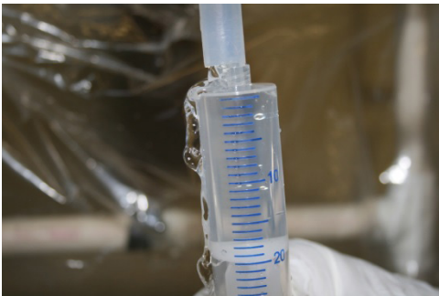
Figure 5.2.2.B-5. Groundwater flowing directly into a syringe. (Photograph taken inside a sample-processing chamber by Michael Manning, U.S. Geological Survey.)
