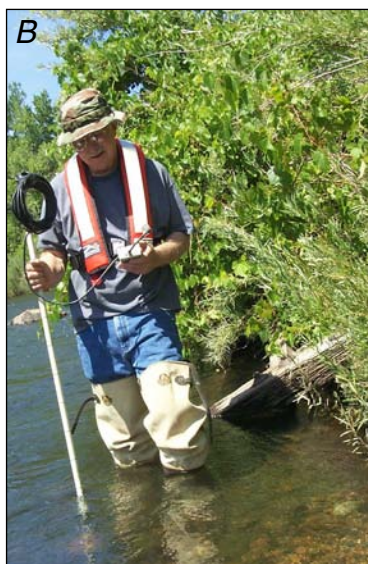
Measuring light penetration using a light meter and light-sensor disk.
