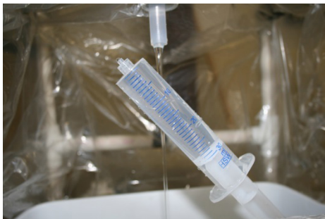
Figure 5.2.2.B–3. Groundwater flowing into a processing chamber is used to rinse the syringe casing. (Photograph by Michael Manning, U.S. Geological Survey.)
